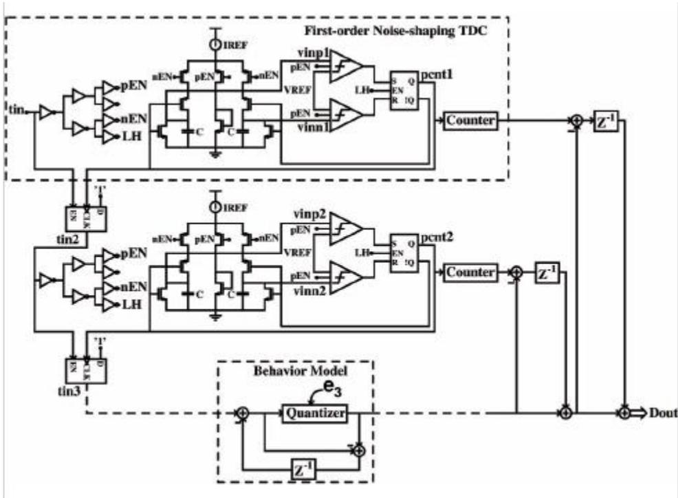
Fig. 5.36 Block diagram of the MASH 1-1-1ΔΣ TDC [11]
