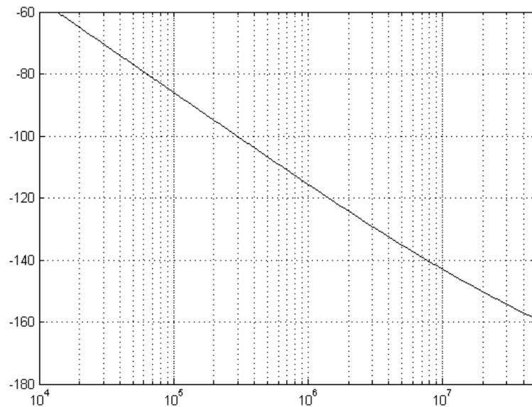
*Fig. 6.32 Behavioral model of the measured free-running DCO phase noise*
