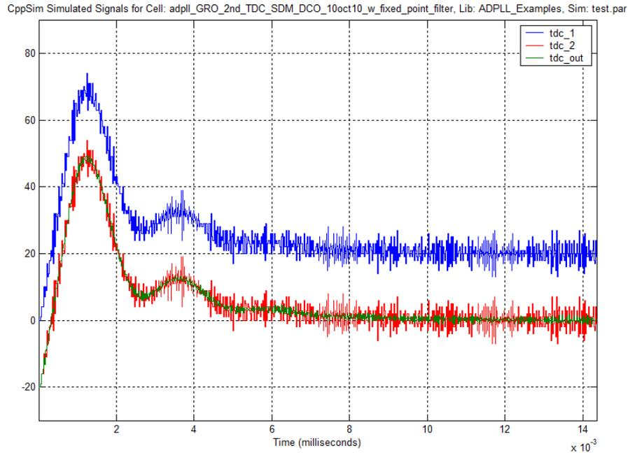
*Fig. 6.14 Transient waveform of the ADPLL (TDC output)*
