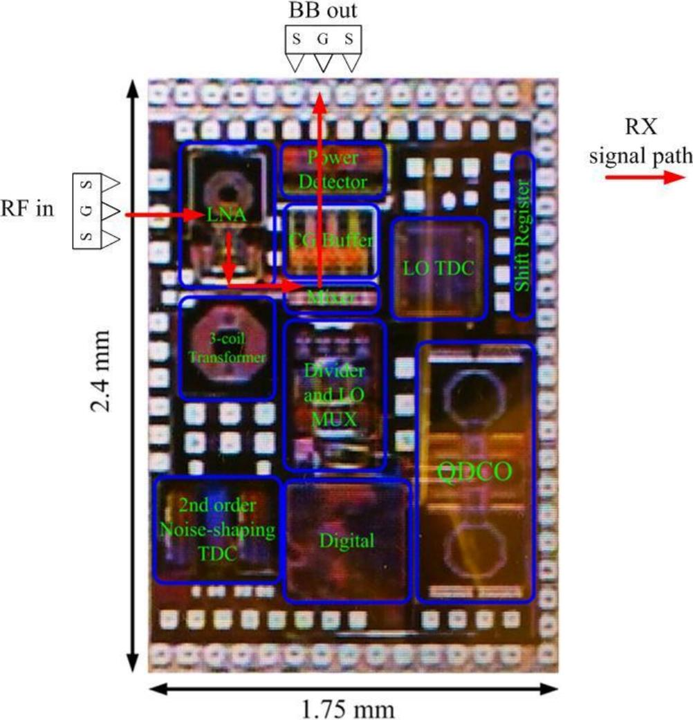
Fig. 8.1 Die micrograph of the receiver front-end
