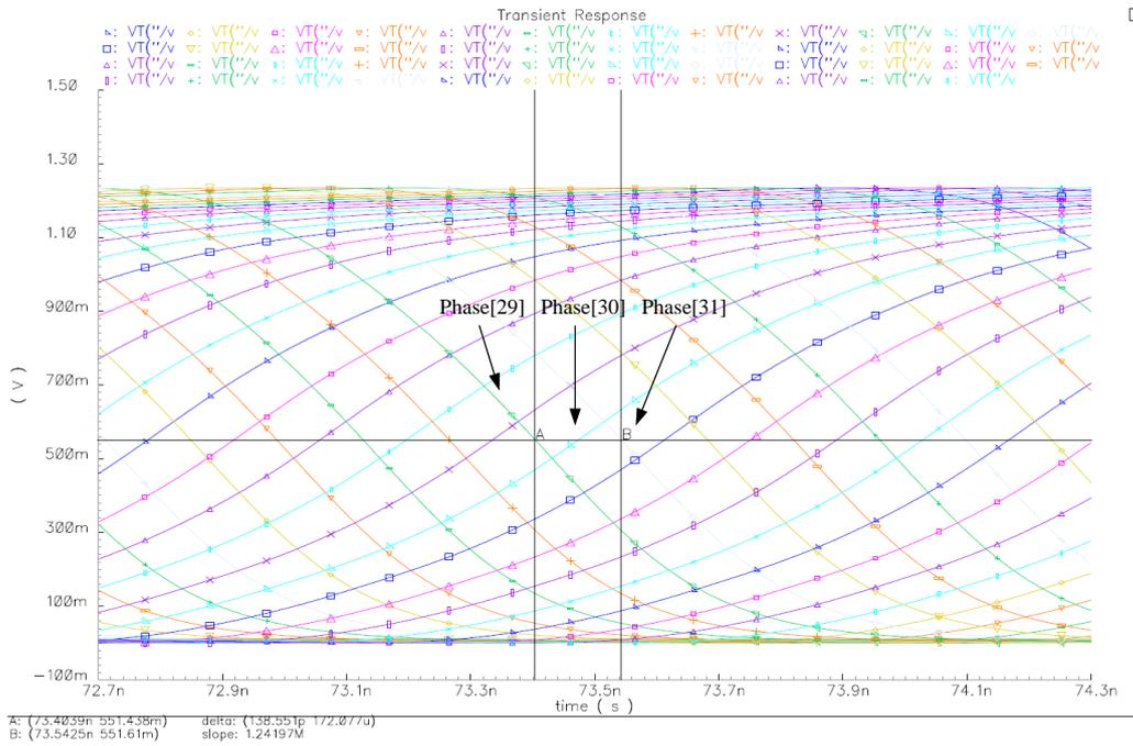
Fig. 5.18 Simulated waveform of single-ended GRO
