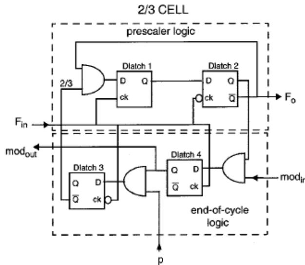
Fig. 6.20 Block Diagram of divide-by-2/3 cell of the programmable divider
