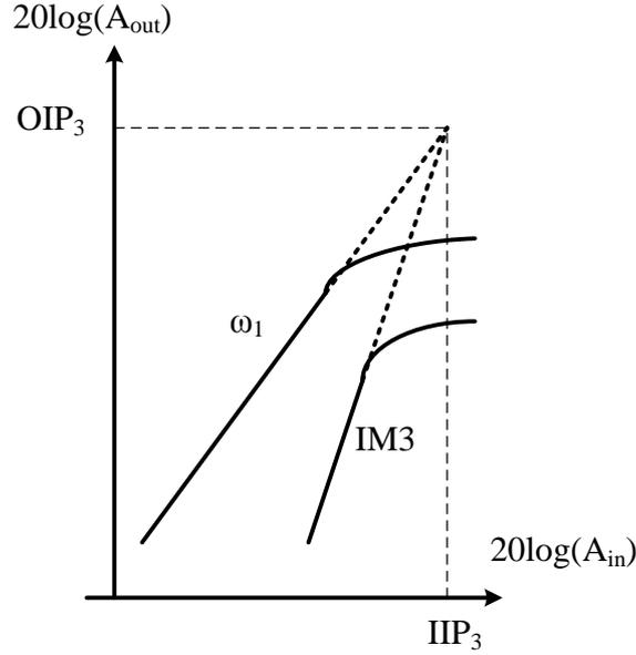
Fig. 2.2 Two-tone test of a non-linear system
