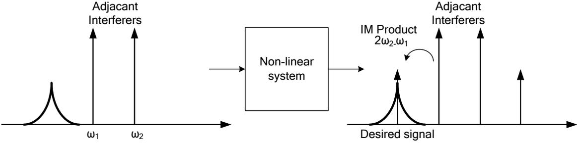
*Fig. 2.1 Corruption of signal due to intermodulation between two interferers*
