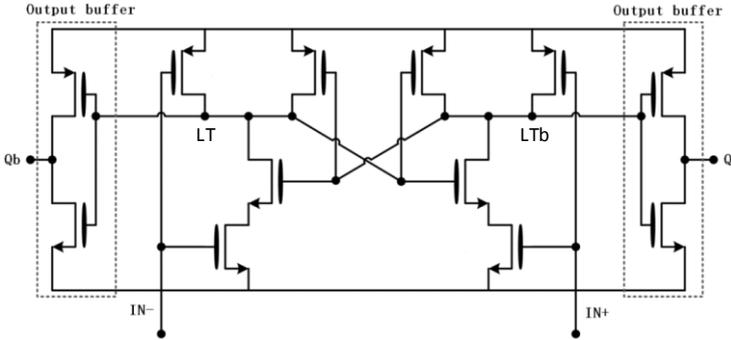
Fig. 7.16 Time comparator for the TDC
