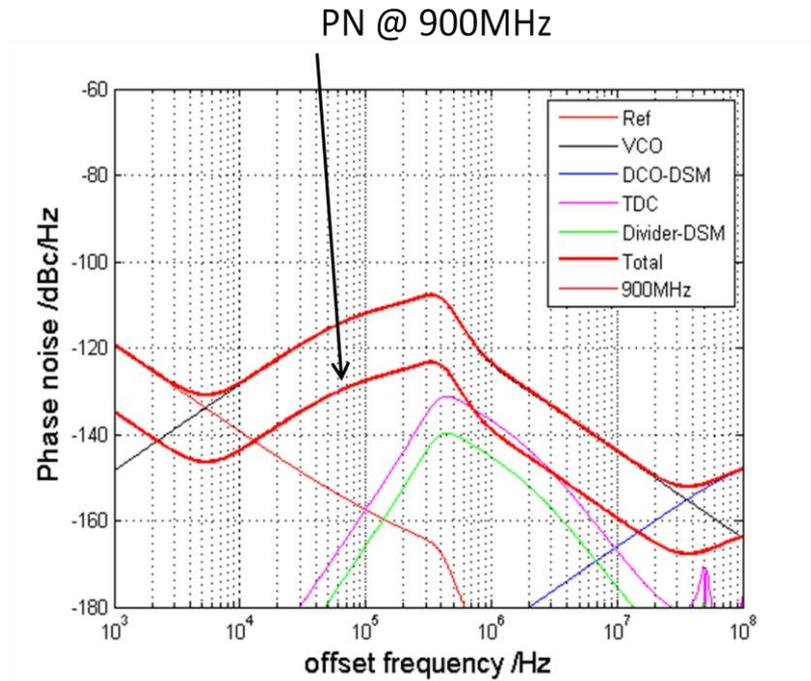
Fig. 6.12 System phase noise plot with output frequency @ 900MHz
