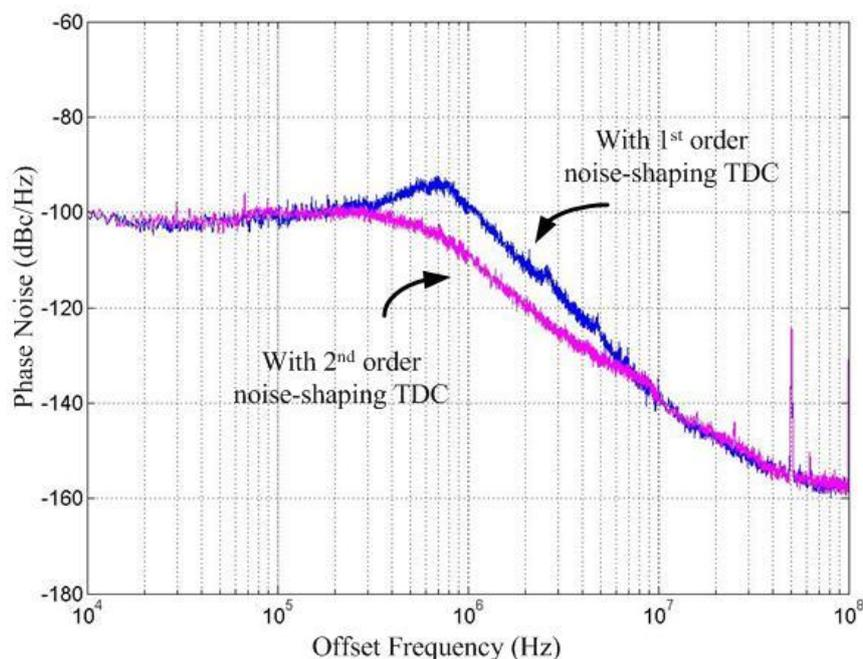
Fig. 6.29 Measured Phase noise plot of the ADPLL with 1<sup>st</sup> and 2<sup>nd</sup> order noise-shaped TDC
