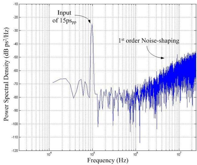
Fig. 5.30 Simulated 1<sup>st</sup> order TDC PSD with GRO phase noise 60ps resolution
