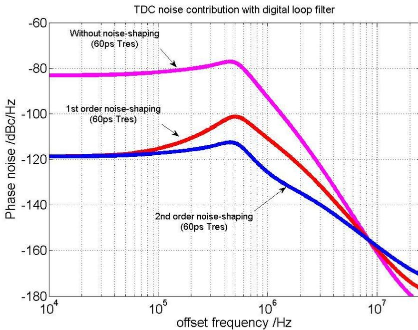
Fig. 5.10 TDC noise contribution being low-pass filtered by PLL transfer function with different TDC order
