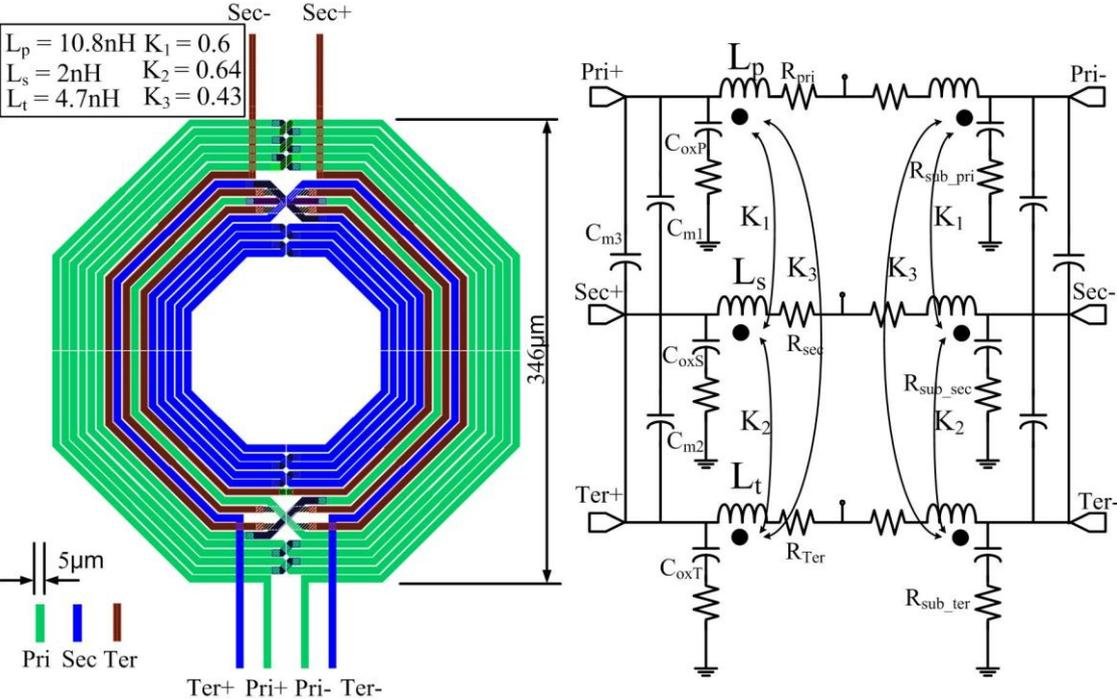
Fig. 7.9 Layout and model of the 3-coils transformer
