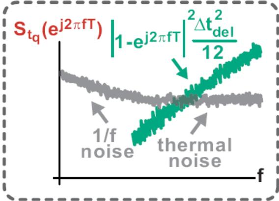
Fig. 5.7 Noise Spectrum of Gated-Ring-Oscillator (GRO) TDC [4]
