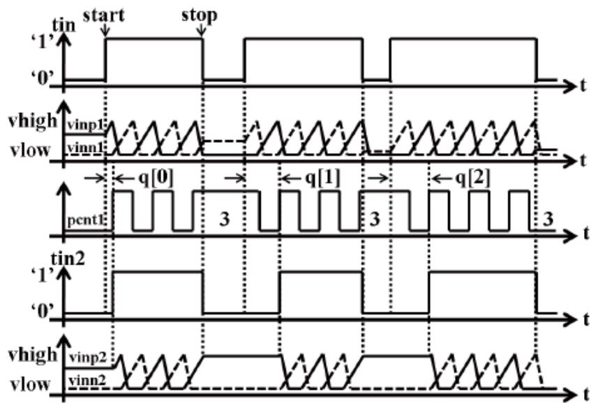
Fig. 5.37 Timing diagram of the MASH 1-1-1ΔΣ TDC [11]
