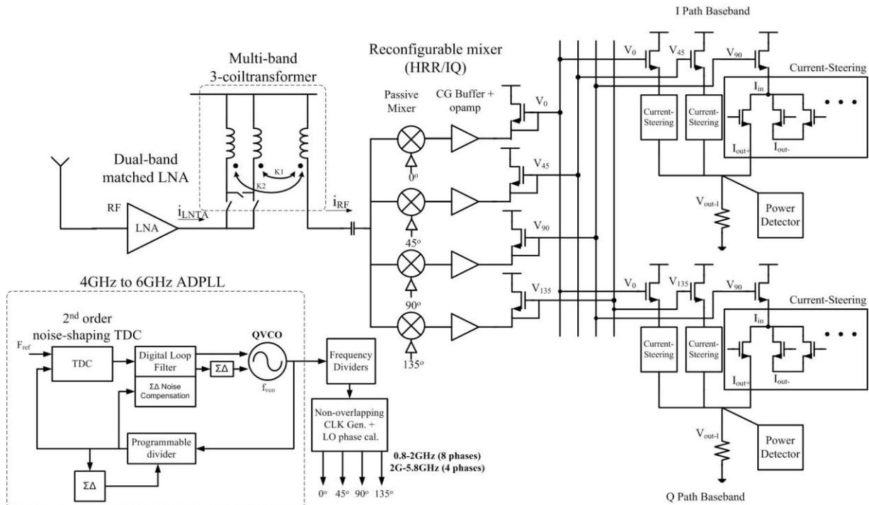
Fig. 1.8 Proposed SDR Receiver Front-End
