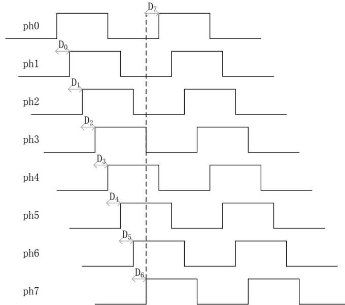
*Fig. 3.12 8-phase to be calibrated*
