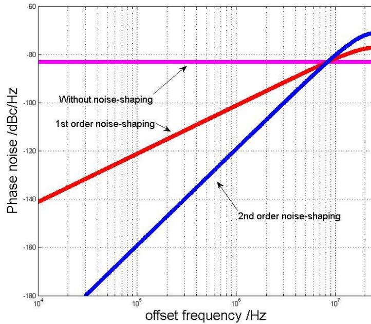
Fig. 6.7 TDC-referred noise power spectral density with different order
