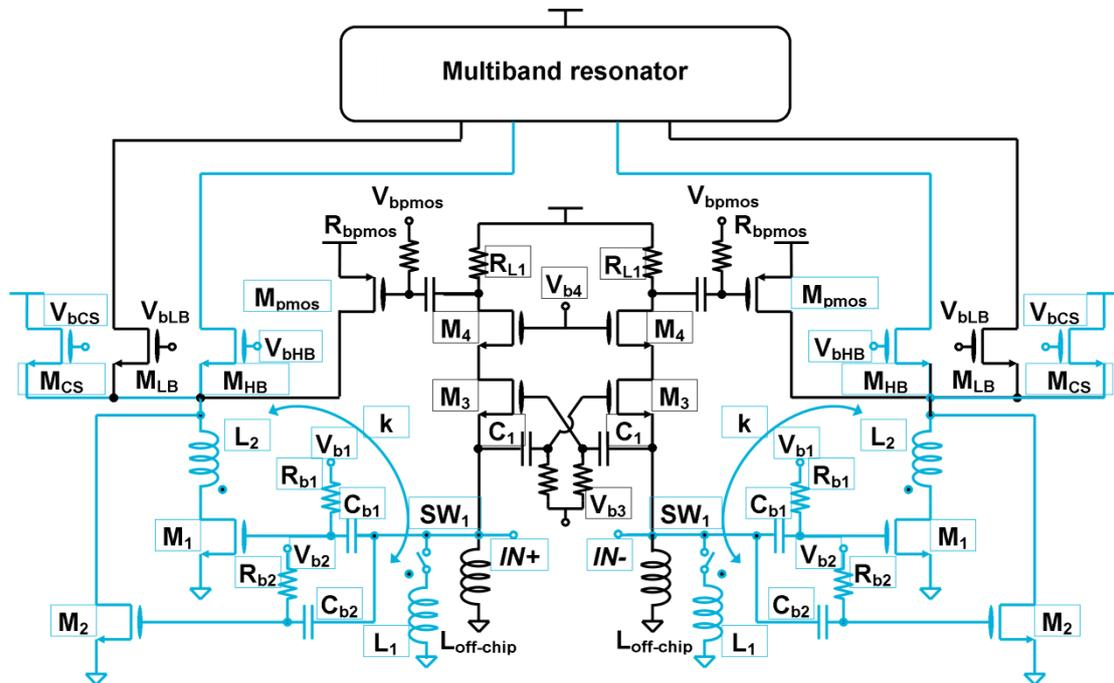
Fig. 7.3 Schematic of the HB LNA
