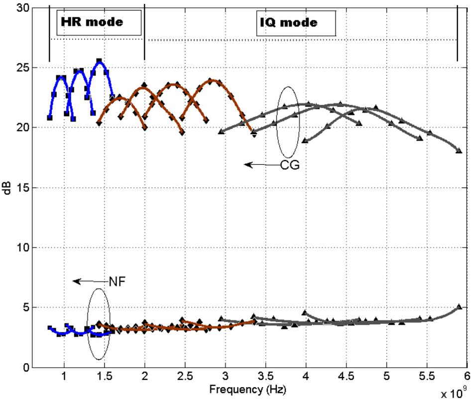
Fig. 8.12 Measured Conversion and DSB NF of the receiver
