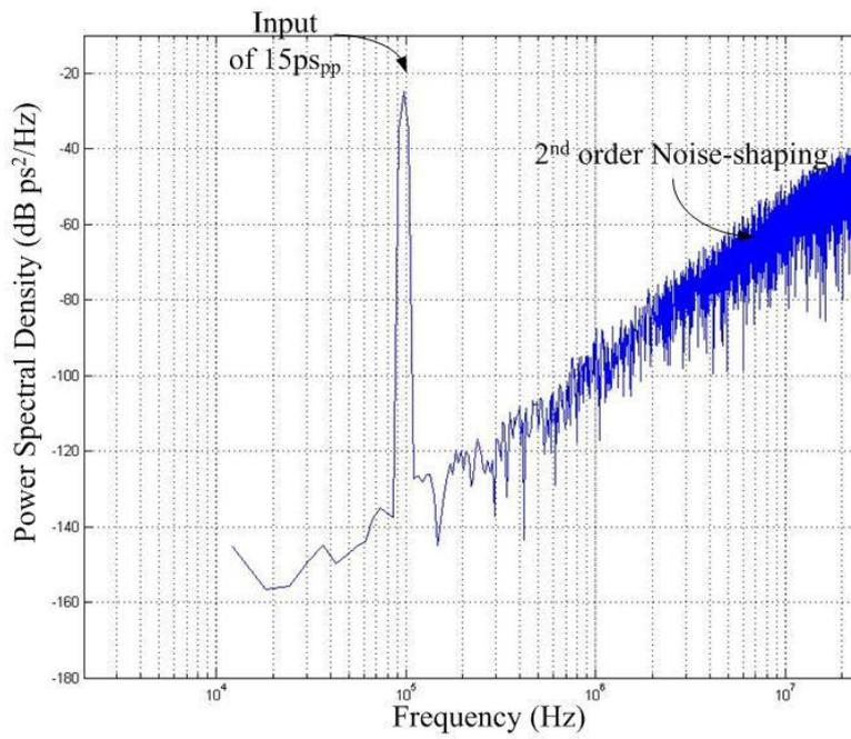
Fig. 5.29 Simulated 2<sup>nd</sup> order TDC PSD without GRO phase noise 60ps resolution
