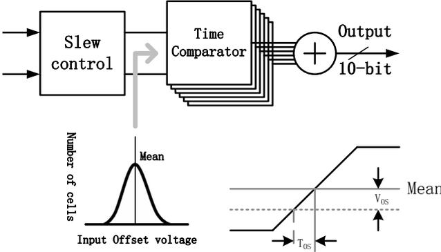
Fig. 7.14 Statistical TDC with gain control
