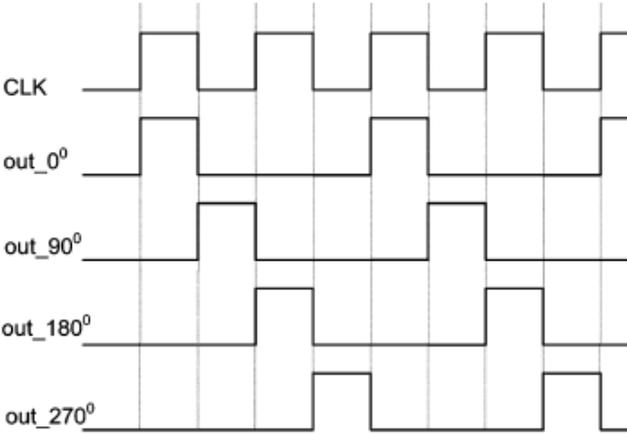
Fig. 3.15 25% duty cycle LO for IQ down-conversion
