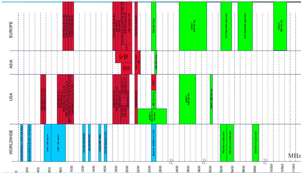
Fig. 1.1 Spectrum allocations of existing wireless standards
