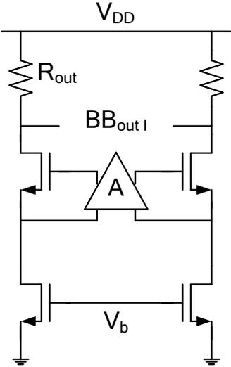
Fig. 7.5 Schematic of the Common-gain current buffer with regulated opamp
