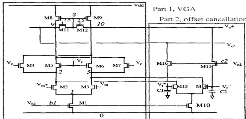
Fig. 7.8 Schematic of the pre-amplifier of the power detector [3]
