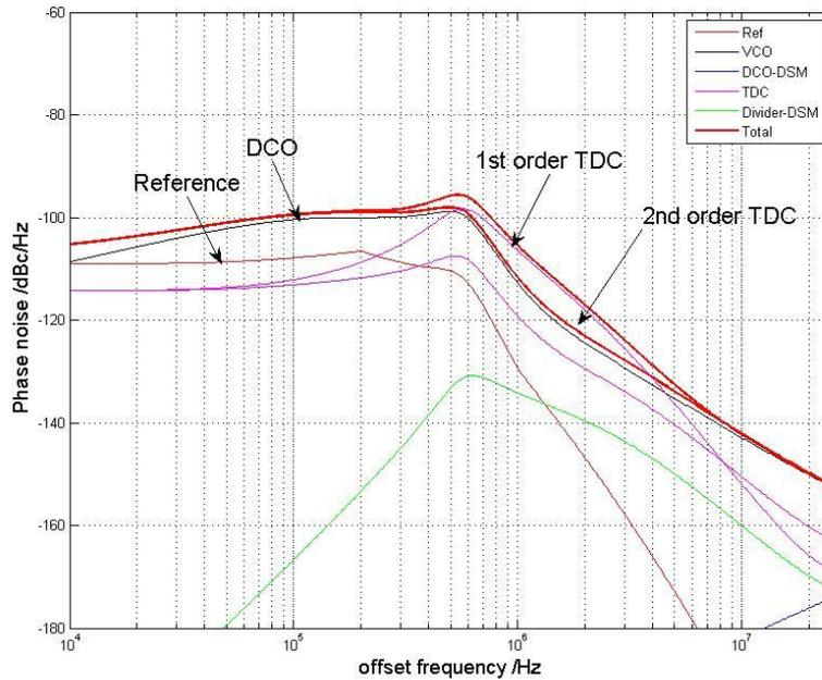
*Fig. 6.33 ADPLL phase noise calculation with measured DCO phase noise*
