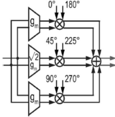
Fig. 3.8 Harmonic-rejection mixer block diagram
