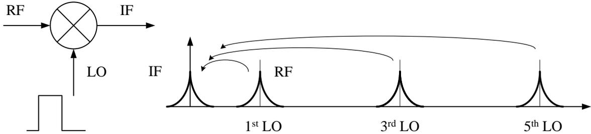
Fig. 2.3 Frequency translation due to hard-switching mixer
