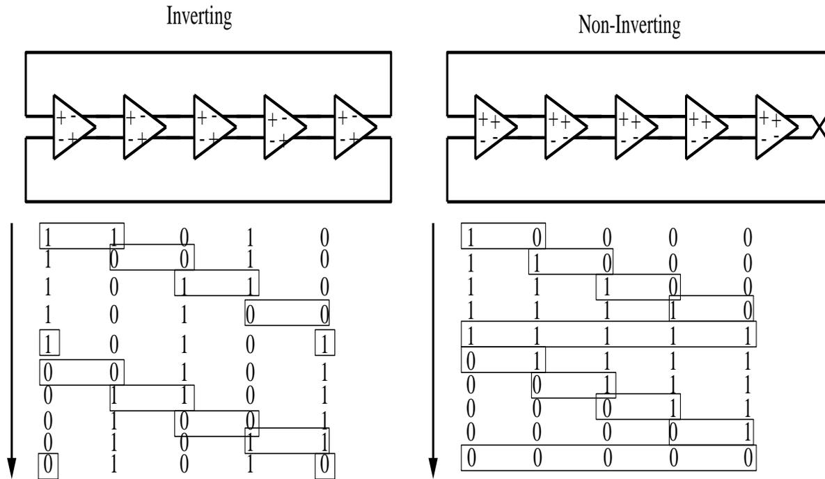
Fig. 5.19 Edge detection of Inverting and Non-Inverting delay cell configuration
