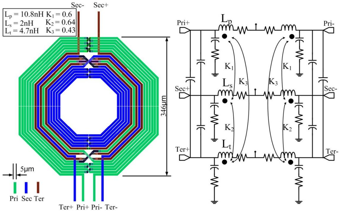
Fig. 4.4 Layout and model of the single 3-coil transformer for the dual-narrow-band RFE
