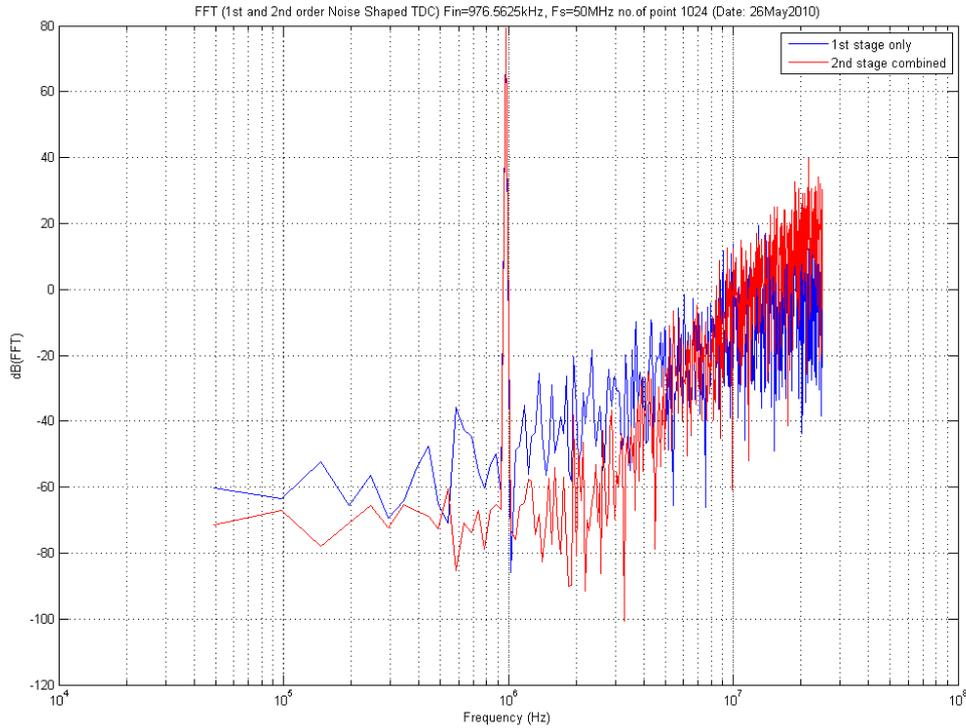
Fig. 5.22 Simulated frequency spectrum of 1<sup>st</sup> and 2<sup>nd</sup> order noise shaped TDC
