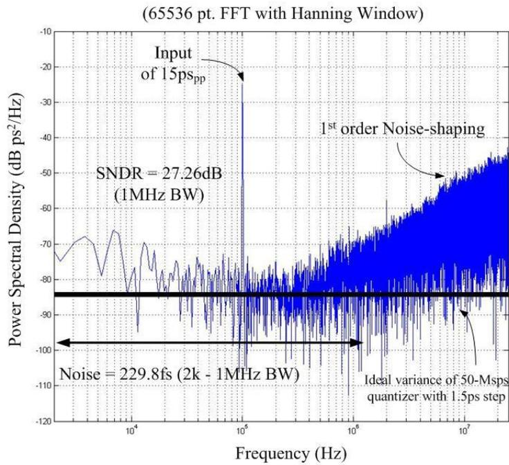
Fig. 5.32 Measured 1<sup>st</sup> order noise-shaping power spectral density with 1.8V GRO Vdd (30ps delay resolution)
