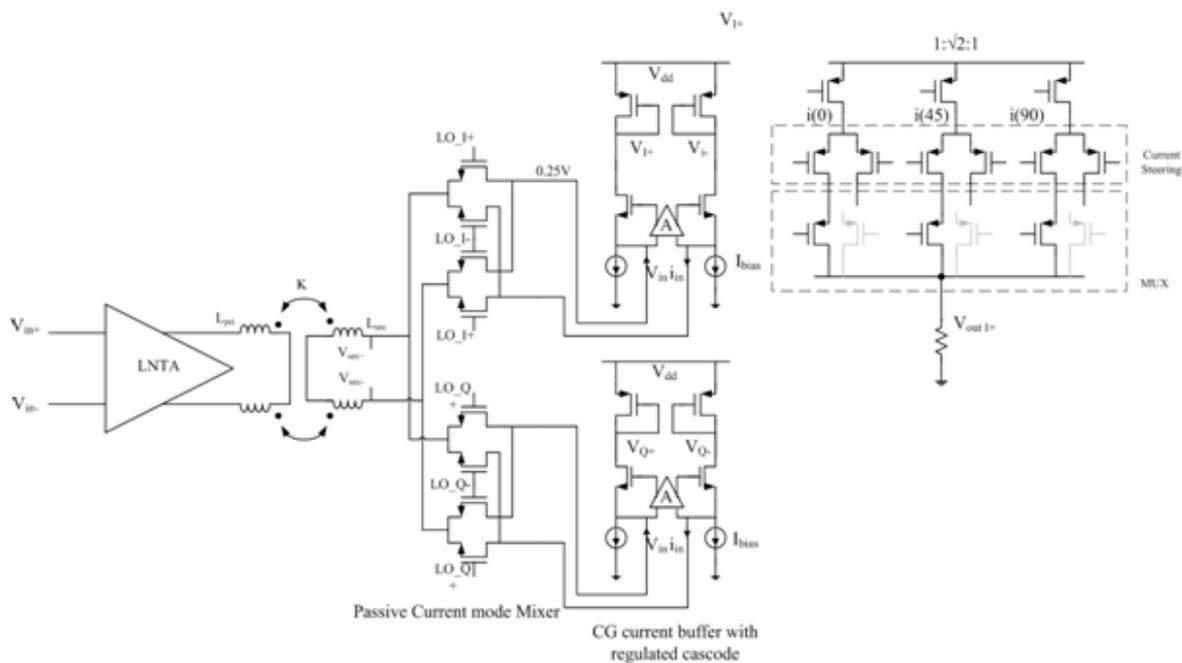
Fig. 7.4 Simplified schematic of the passive current-driven mixer with current steering baseband for fine gain tuning
