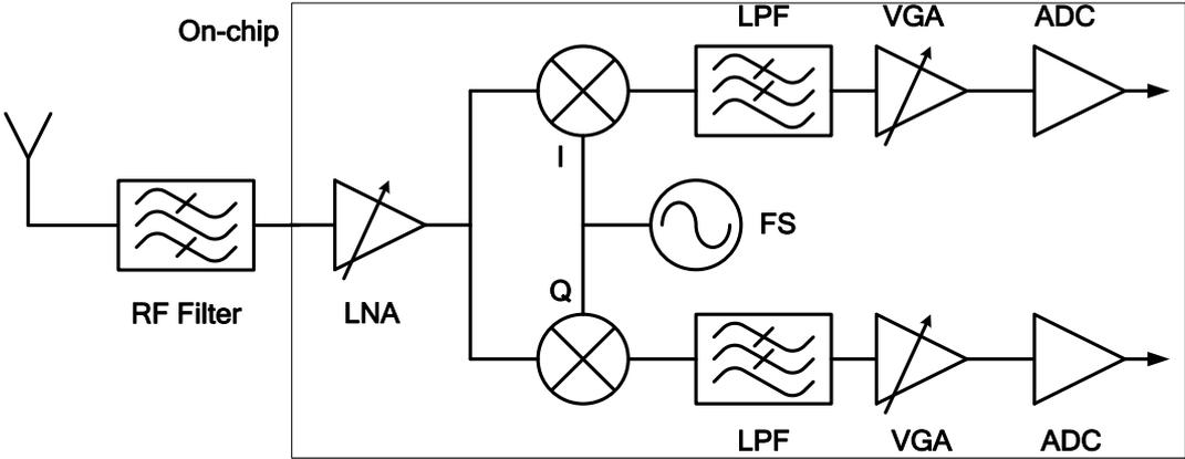
Fig. 1.4 Direct-Conversion Receiver Architecture
