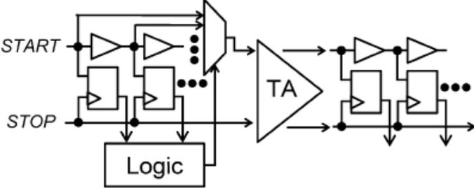
Fig. 7.13 Two-step TDC with time amplifier
