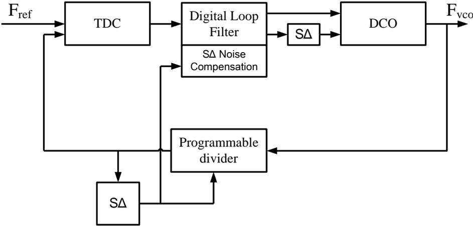
Fig. 5.2 All-Digital Phase-Locked Loop
