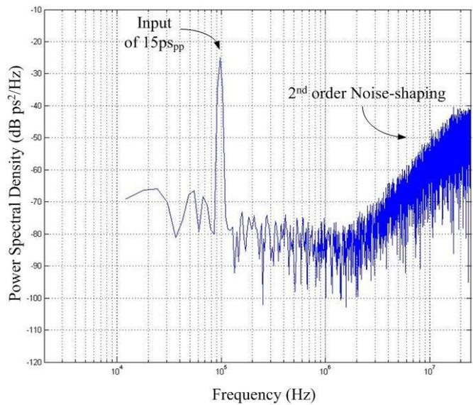
Fig. 5.31 Simulated 2<sup>nd</sup> order TDC PSD without GRO phase noise 60ps resolution
