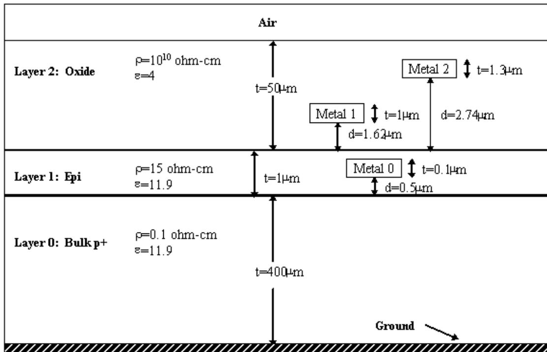
Fig. 7.10 Typical Substrate Profile ( From ASITIC Software Manual )
