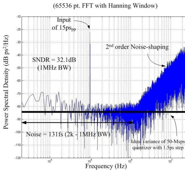
Fig. 5.33 Measured 2<sup>nd</sup> order noise-shaping power spectral density with 1.8V GRO Vdd (30ps delay resolution)
