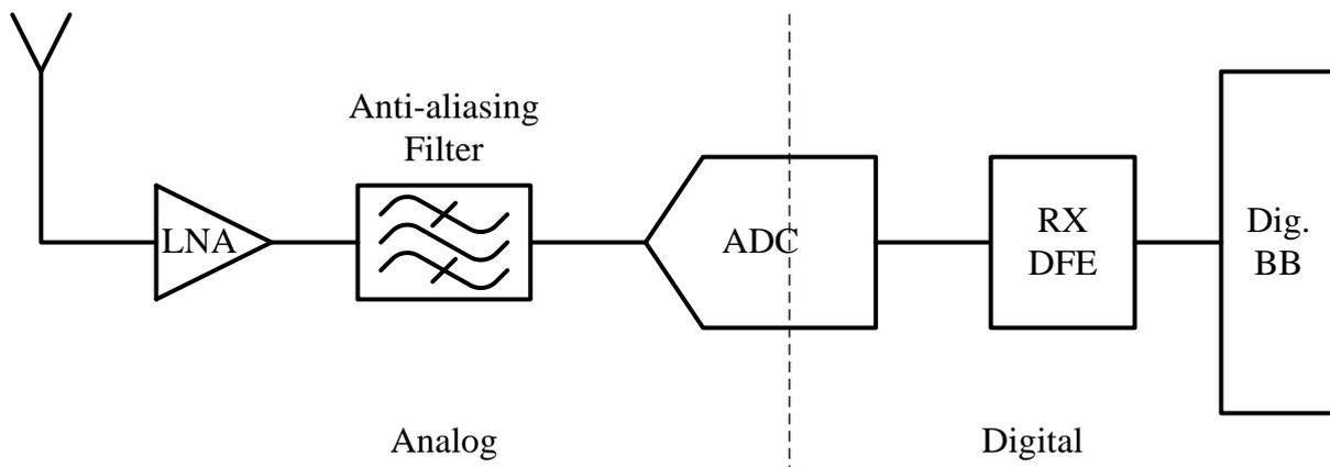
*Fig. 3.1 Ideal SDR receiver architecture*
