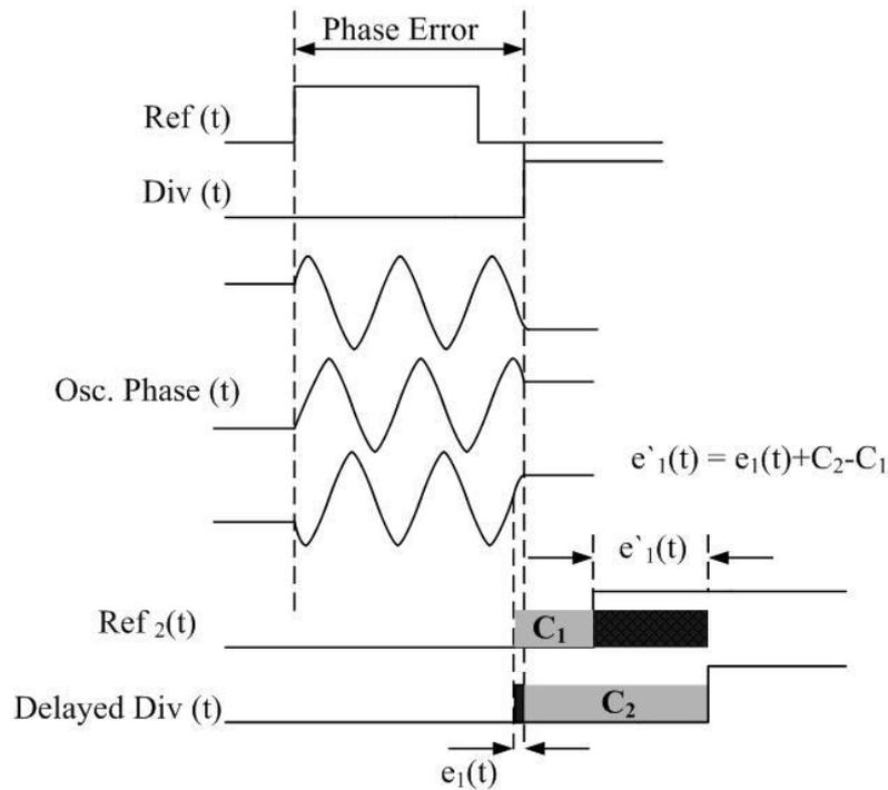
Fig. 5.16 Timing diagram for the residue extraction
