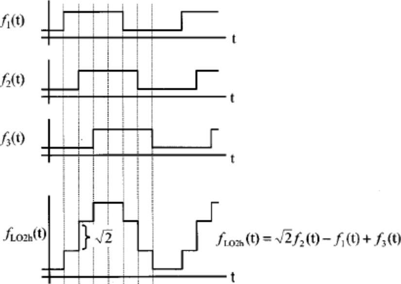
Fig. 3.7 Harmonic-rejection signal generation [5]
