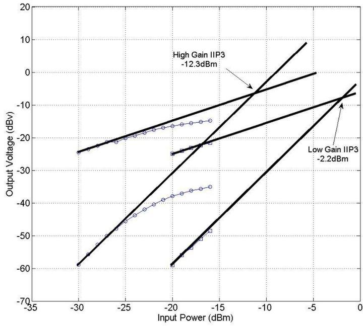
Fig. 8.14 Measured Low-band IIP3 at Low-Gain and High-Gain setting
