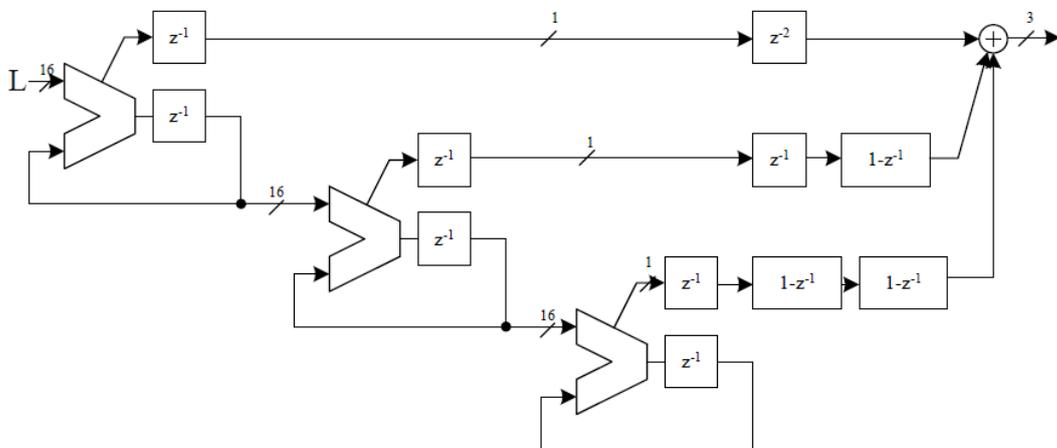
Fig. 6.22 MASH 1-1-1 SDM for the Programmable Divider
