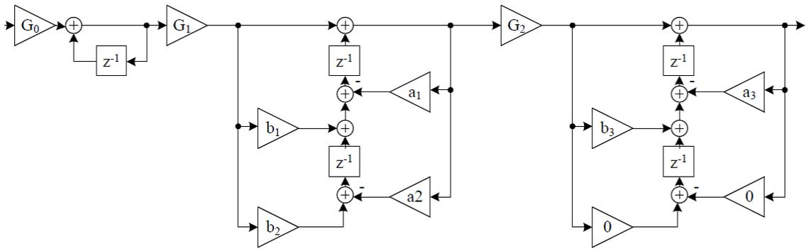
Fig. 6.21 FIR Digital Loop Filter (Cascade of Biquad Filter Structure)
