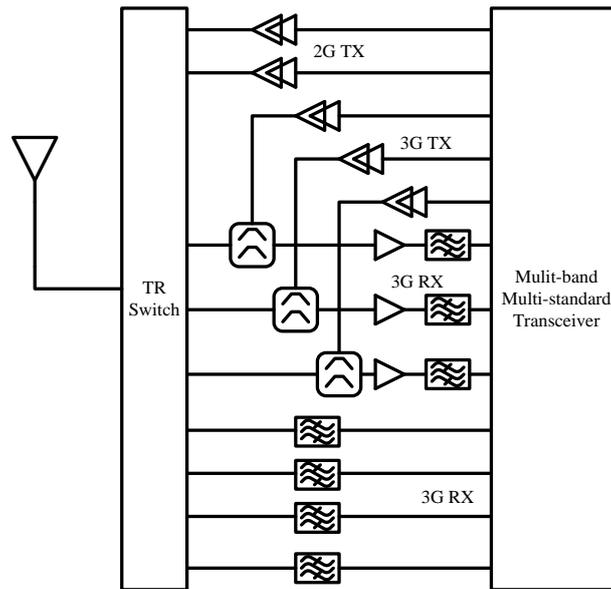
*Fig. 1.5 Example of existing multi-band multi-standard transceiver*
