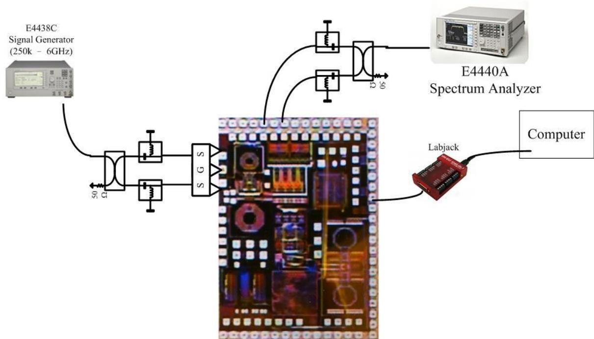
Fig. 8.5 Measurement setup for the receiver.
