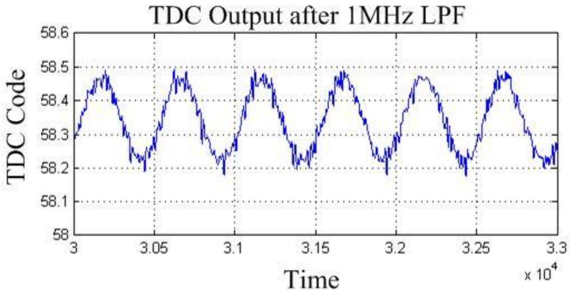
*Fig. 5.26 Measured 2<sup>nd</sup> order noise-shaping waveform after 1MHz LPF*
