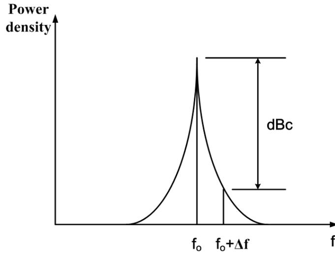
Fig. 2.4 Frequency spectrum of a real oscillator
