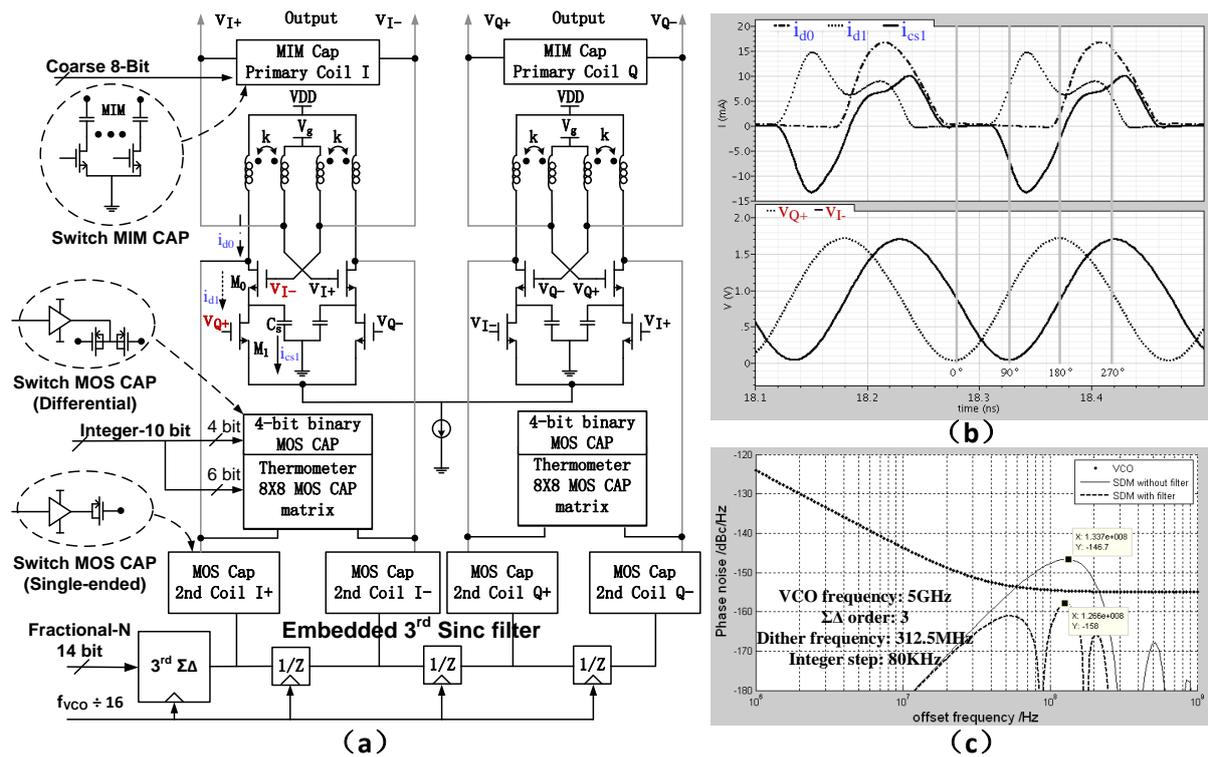
Fig. 6.18(a) Schematic of the QDCO (b) Oscillation waveform (c) Phase Noise (Courtesy of Mr. Zheng Shi Yuan)
