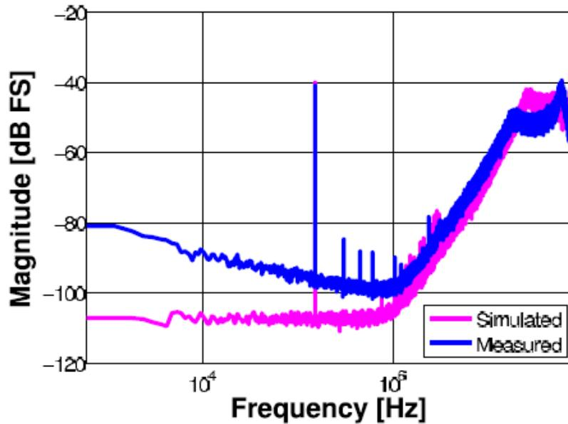
Fig. 5.35 Measured spectrum of the continuous-time  $\Delta\Sigma$  TDC [10]
