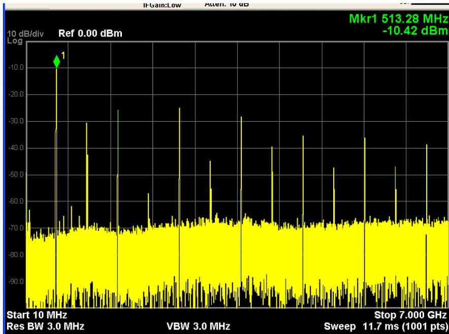
Fig. 8.10 Measured output spectrum of the LO with minimum output frequency @ 512MHz
