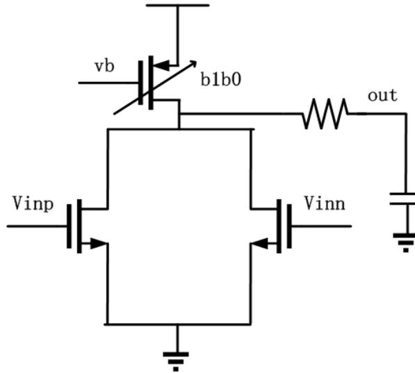
Fig. 7.7 Power Detector Circuitry
