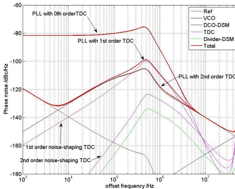
Fig. 6.9 Calculated phase noise contribution for the ADPLL with different order TDC
