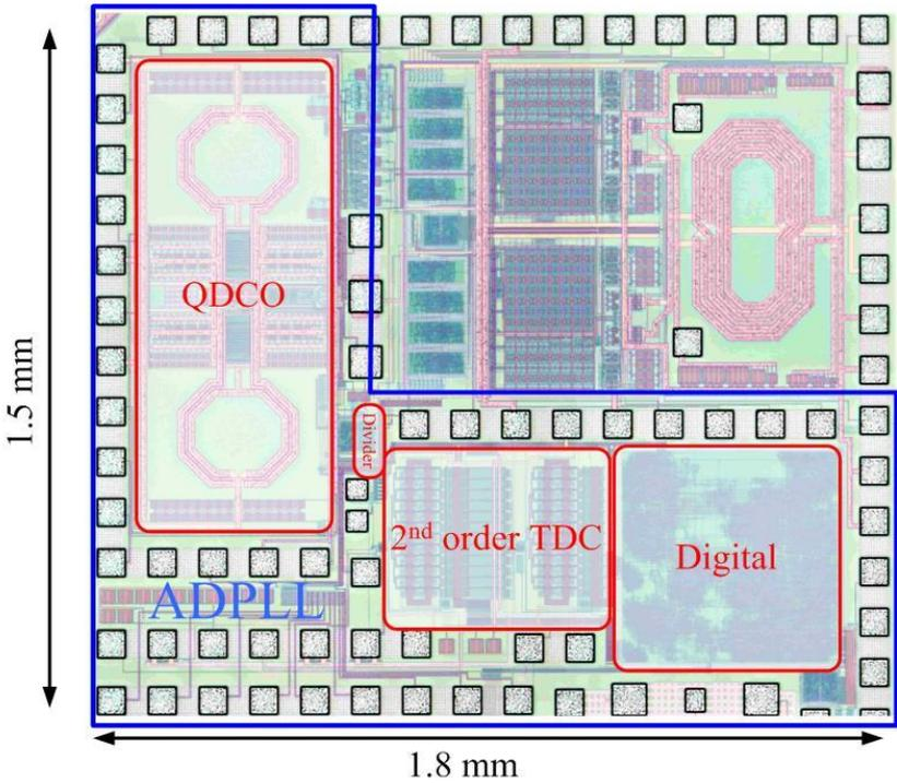
Fig. 6.23 Die Micrograph of the ADPLL (part of SDR Transmitter)
