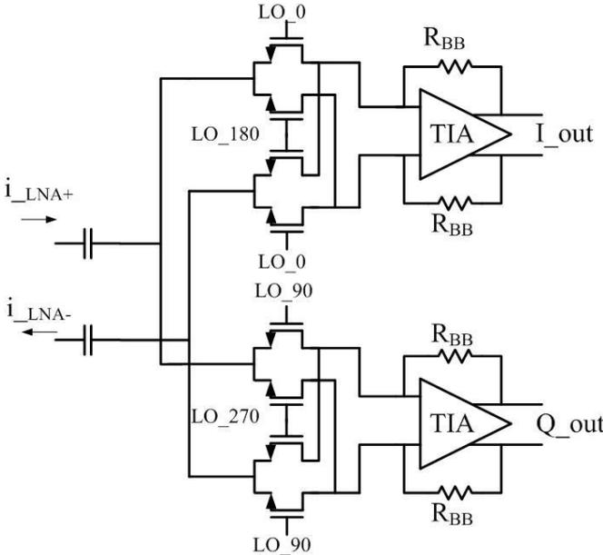
Fig. 3.14 Passive current-driven IQ mixer
