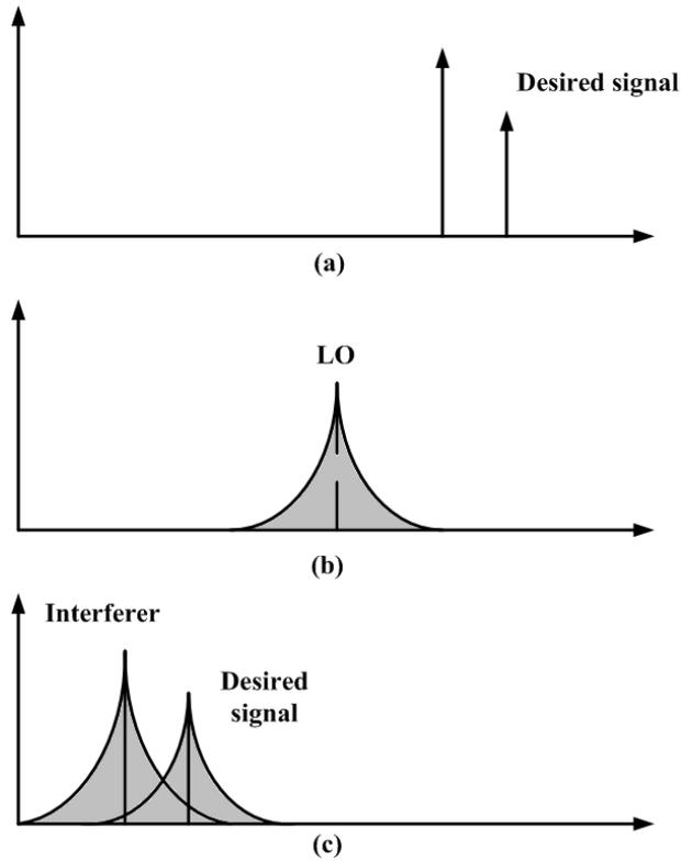
Fig. 2.6 Effect of phase noise in a receiver in the presence of phase noise
