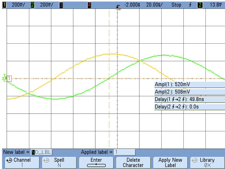
Fig. 8.23 Time domain waveform at IF output with LO phase calibration ( $RF = 1.5\text{GHz}$ ,  $LO = 1.45\text{GHz}$ ,  $IF = 5\text{MHz}$ )
