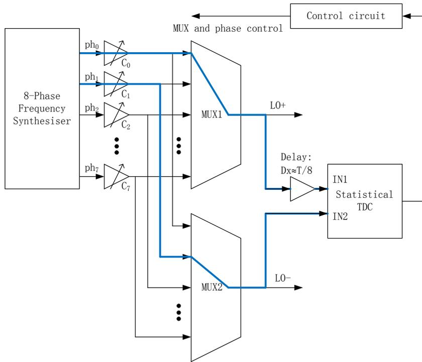
Fig. 3.11 Blocks diagram of the phase selection and calibration
