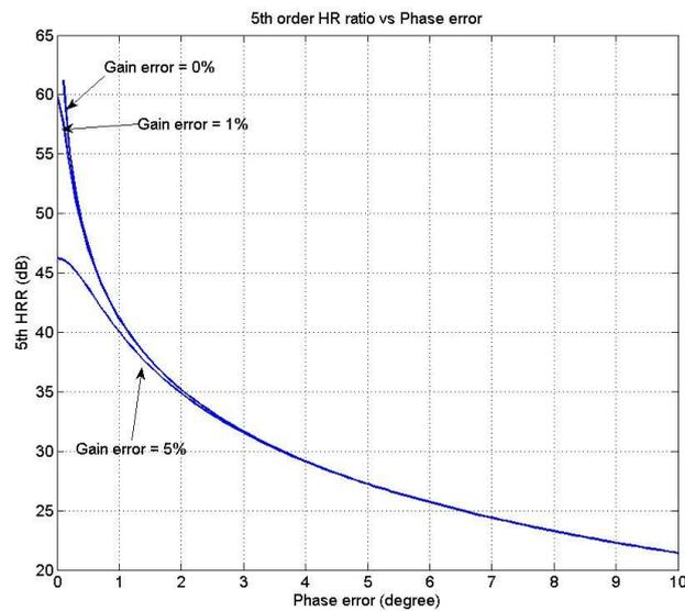
Fig. 8.19 Calculated HR5 as a function of phase error for various gain errors
