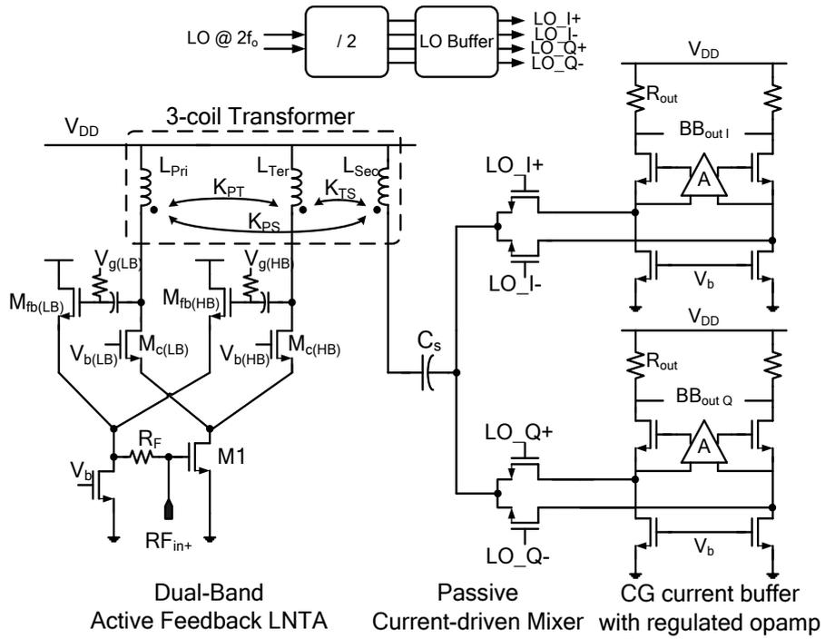
Fig. 4.2 Current-gain-boost low-noise dual-narrow-band RFE with a 3-coil differential transformer (In actual implementation, LNTA is differential and the mixer are double-balanced)
