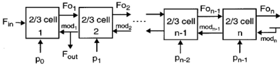
Fig. 6.19 Block Diagram of the programmable divider
