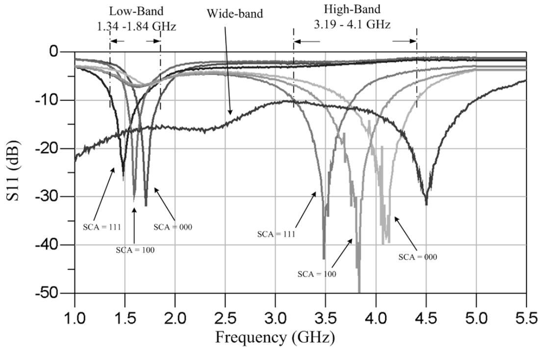
Fig. 4.6 Measured  $S_{11}$  of the dual-narrow-band and the wide-band RFEs
