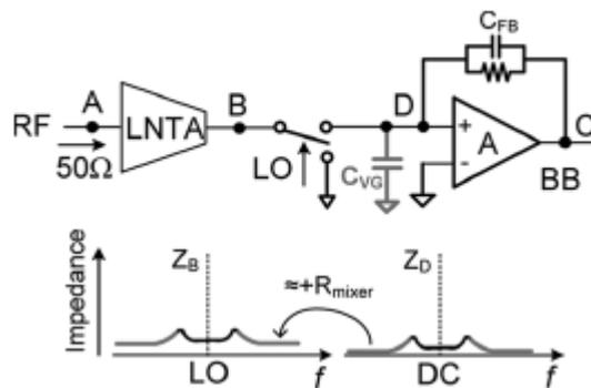
Fig. 1.6 Blocker filtering using impedance transfer [4]
