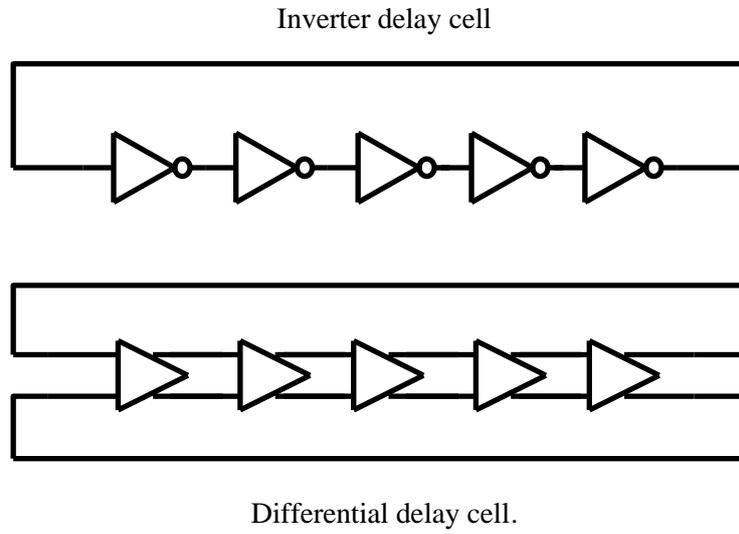
Fig. 5.17 Single-ended and Differential delay-cell configuration
