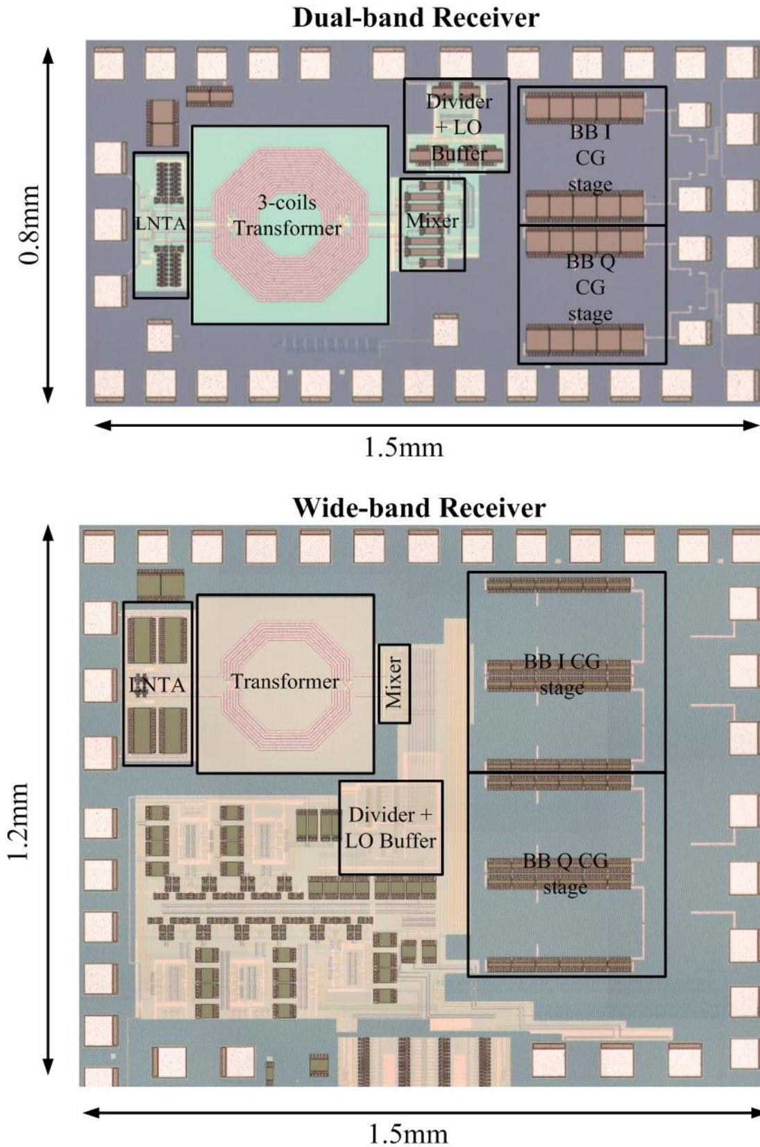
*Fig. 4.5 Die micrographs of the dual-narrow-band and wide-band RFEs*
