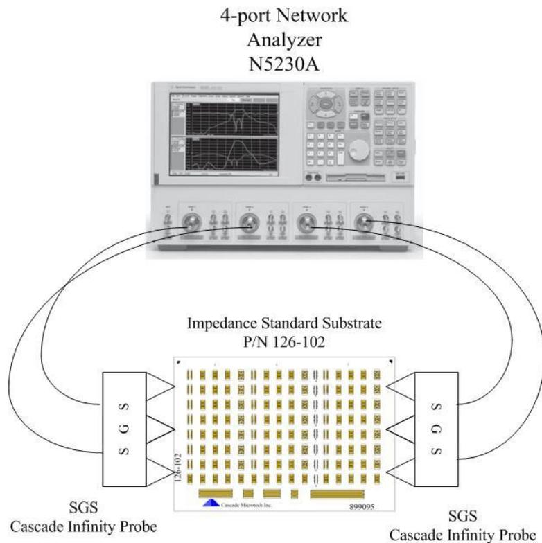
*Fig. 8.6 Calibration setup of the 4-port network analyzer (N5230A)*
