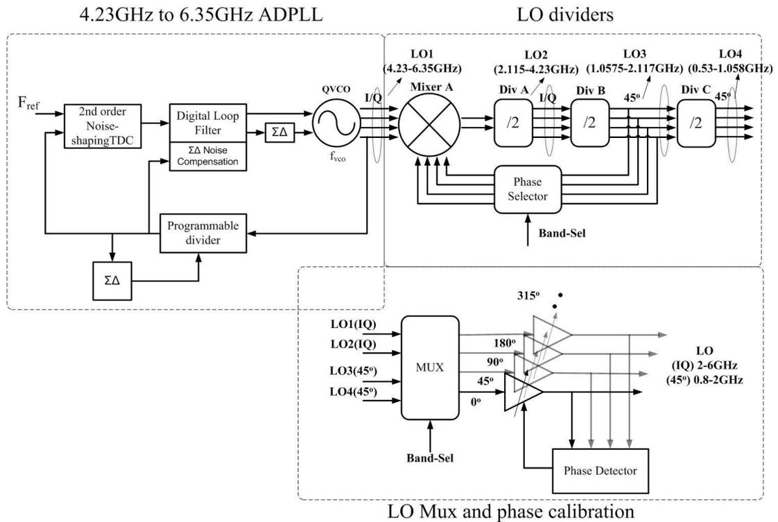
Fig. 6.1 Block diagram of the LO generation system for the SDR RFE
