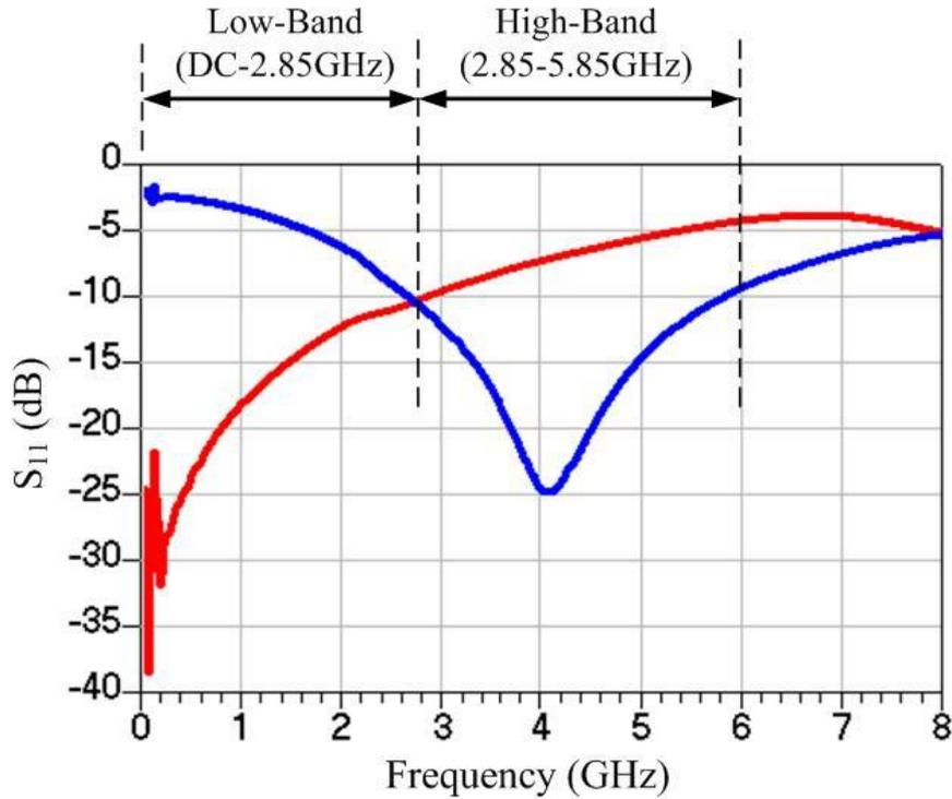
Fig. 8.11 Measured  $S_{11}$  of the receiver
