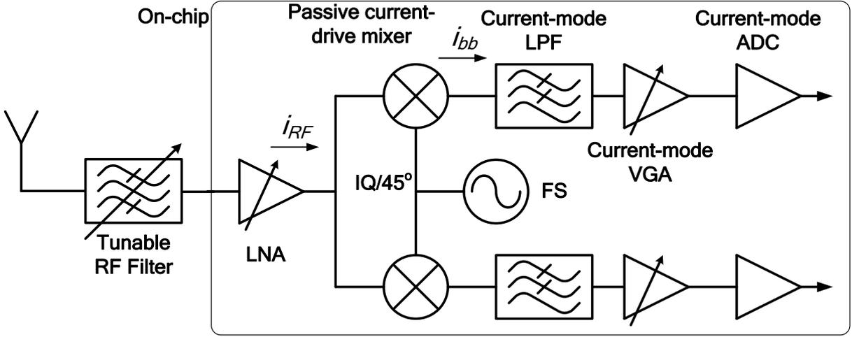
Fig. 9.1 Block diagram of a current-mode RFE
