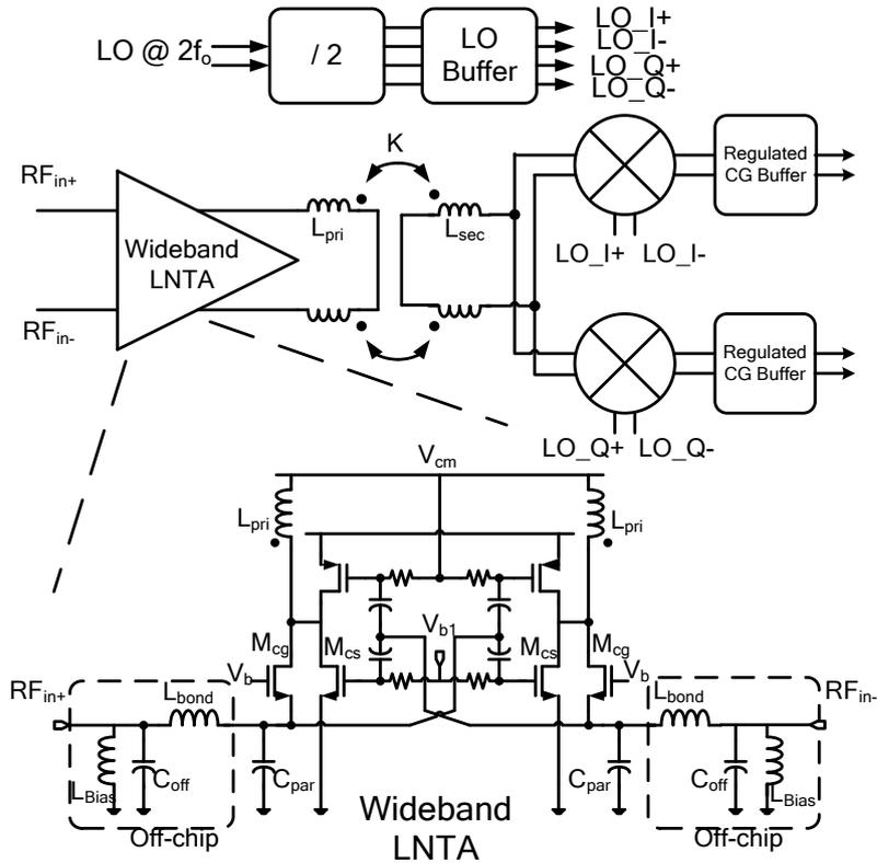
Fig. 4.3 Current-gain-boost high-linearity wide-band RFE
