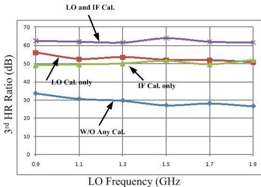
Fig. 8.20 Measured 3<sup>rd</sup> order HR ratio (HRR mixer only) versus LO frequency
