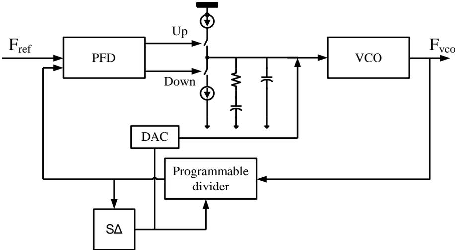
Fig. 5.1 Conventional Charge-Pump Phase-Locked Loop
