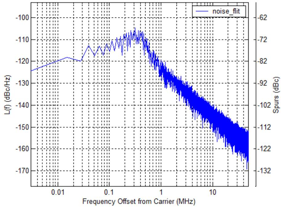
Fig. 6.15 Phase noise plot at Cppsim after transient simulation
