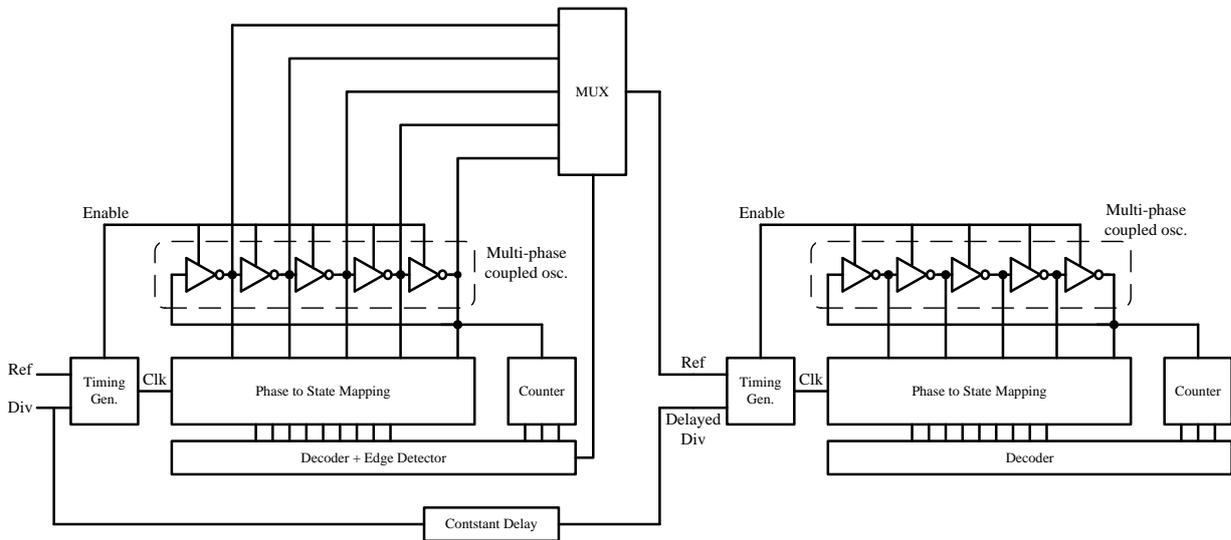
Fig. 6.17 Block diagram of the 2<sup>nd</sup> order noise-shaped TDC
