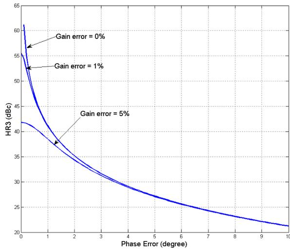
Fig. 8.18 Calculated HR3 as a function of phase error for various gain errors
