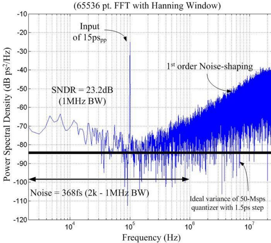
Fig. 5.24 Measured 1<sup>st</sup> order noise-shaping power spectral density
