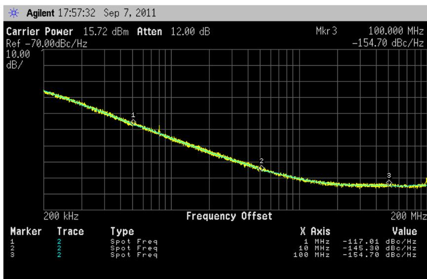
Fig. 6.27 measured free-running phase noise of the DCO
