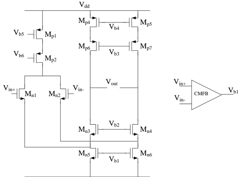
Fig. 7.6 Schematic of a folded cascade opamp
