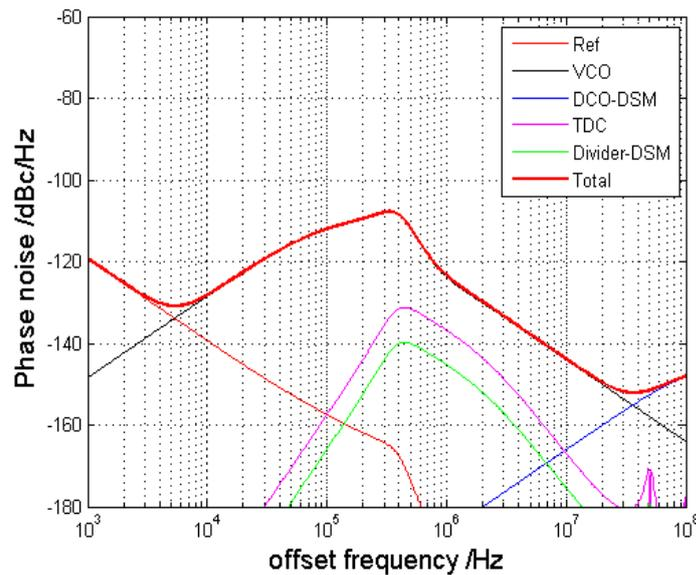
Fig. 6.11 System phase noise plot with output frequency at 5.4GHz
