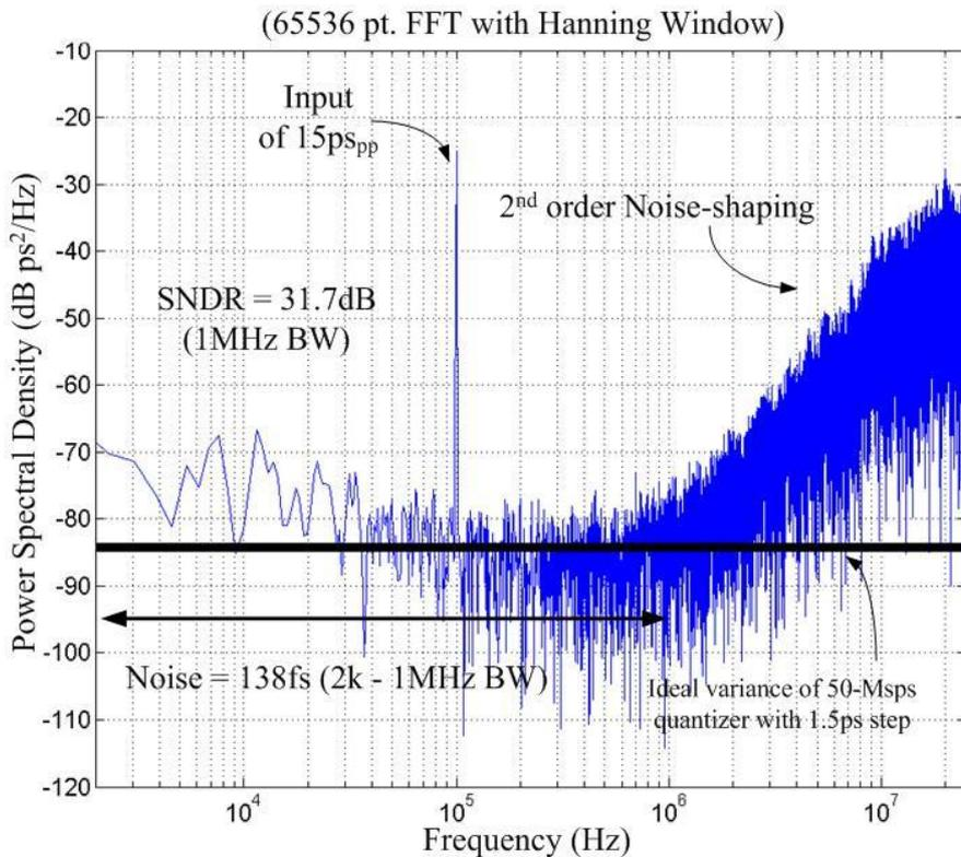
Fig. 5.25 Measured 2<sup>nd</sup> order noise-shaping power spectral density
