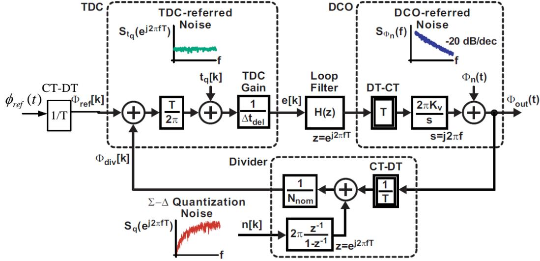
Fig. 6.6 Model of ADPLL with different noise sources [1].
