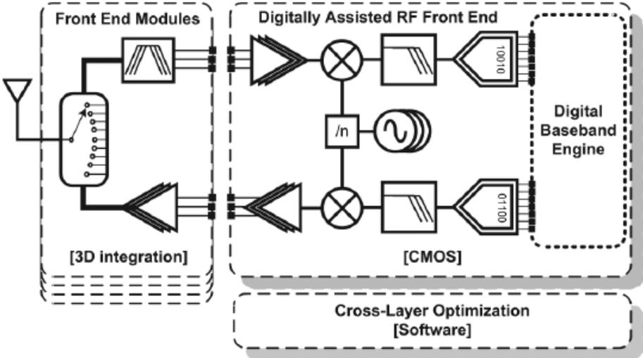
Fig. 1.7 SDR platform proposed in [5], requiring a multiple front-end modules and a analog RFE.
