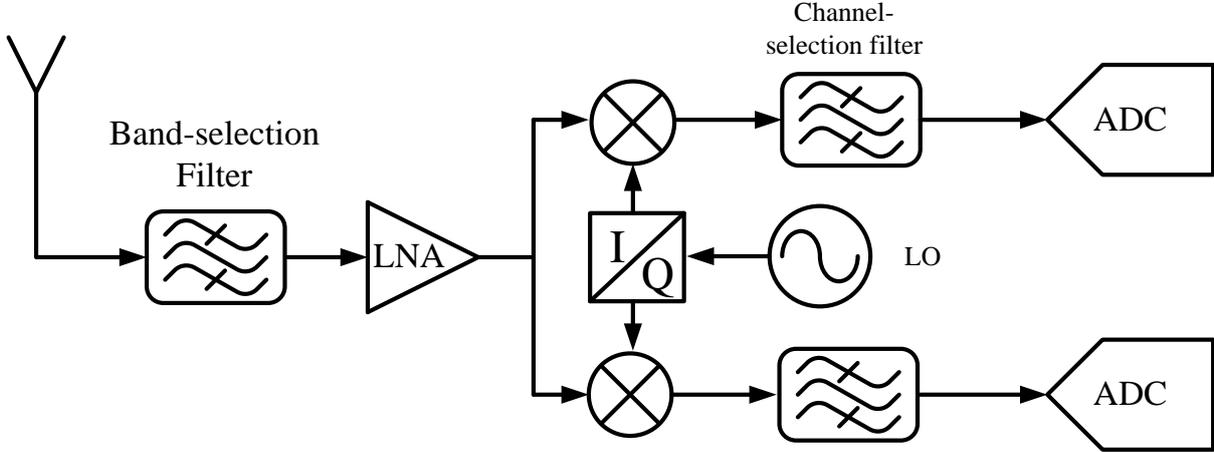
Fig. 3.4 Direct-conversion receiver
