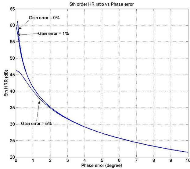
Fig. 3.10 Calculated HR5 as a function of phase error for various gain errors
