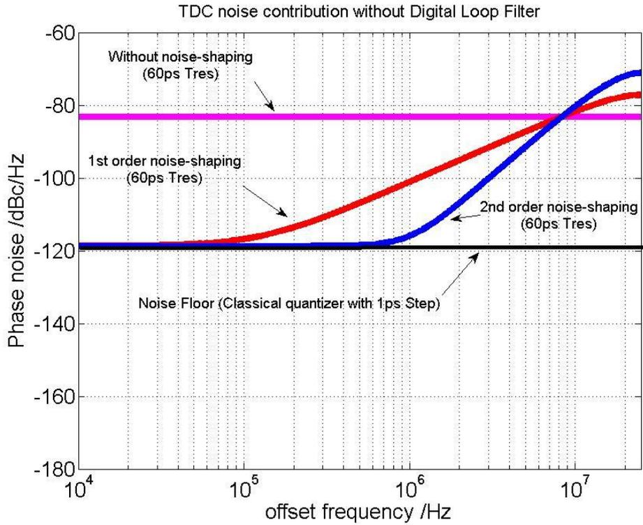
Fig. 5.9 TDC quantization noise contribution to ADPLL with different noise-shaping order
