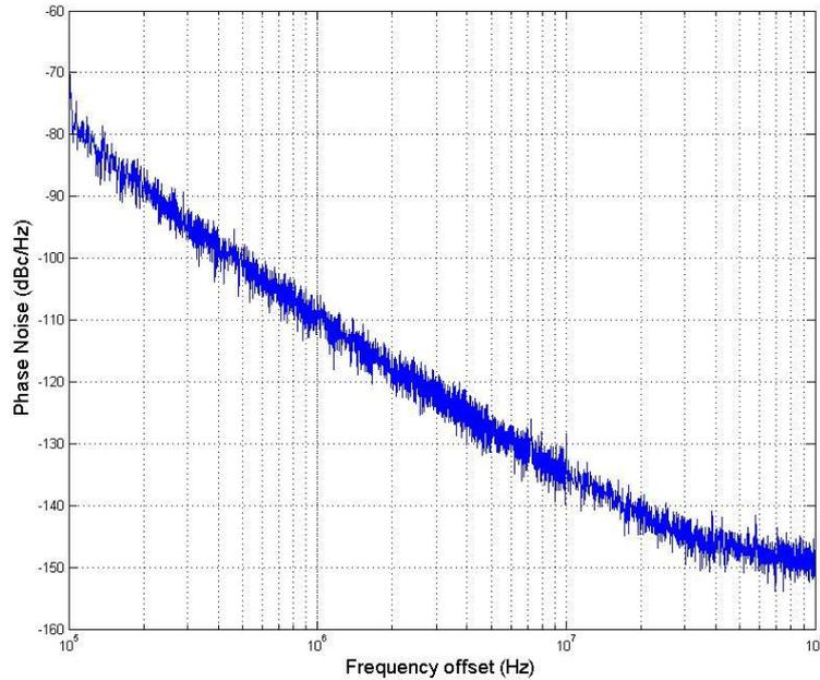
*Fig. 5.27 Measured phase noise of the multi-path coupled oscillator inside the GRO TDC*
