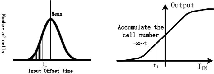
Fig. 7.15 Time offset distribution and TDC input-output characteristic
