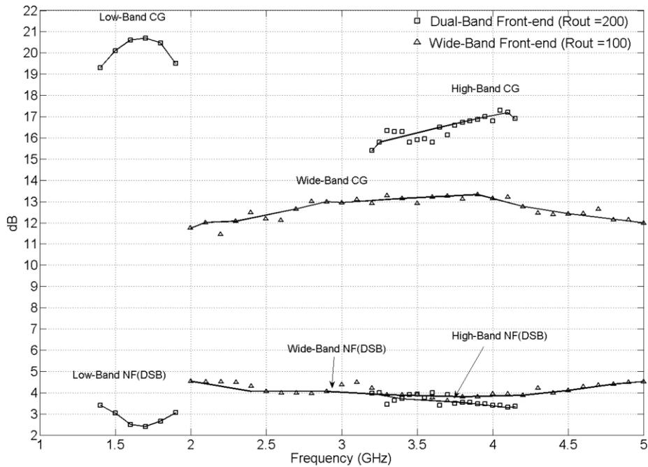
Fig. 4.7 Measured gains and NF of the dual-narrow-band and the wide-band RFEs
