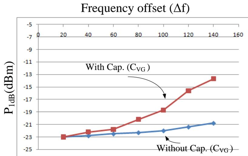
Fig. 8.15 Measured low-band  $P_{1dB}$  with RF located at  $f_{LO} + \Delta f$
