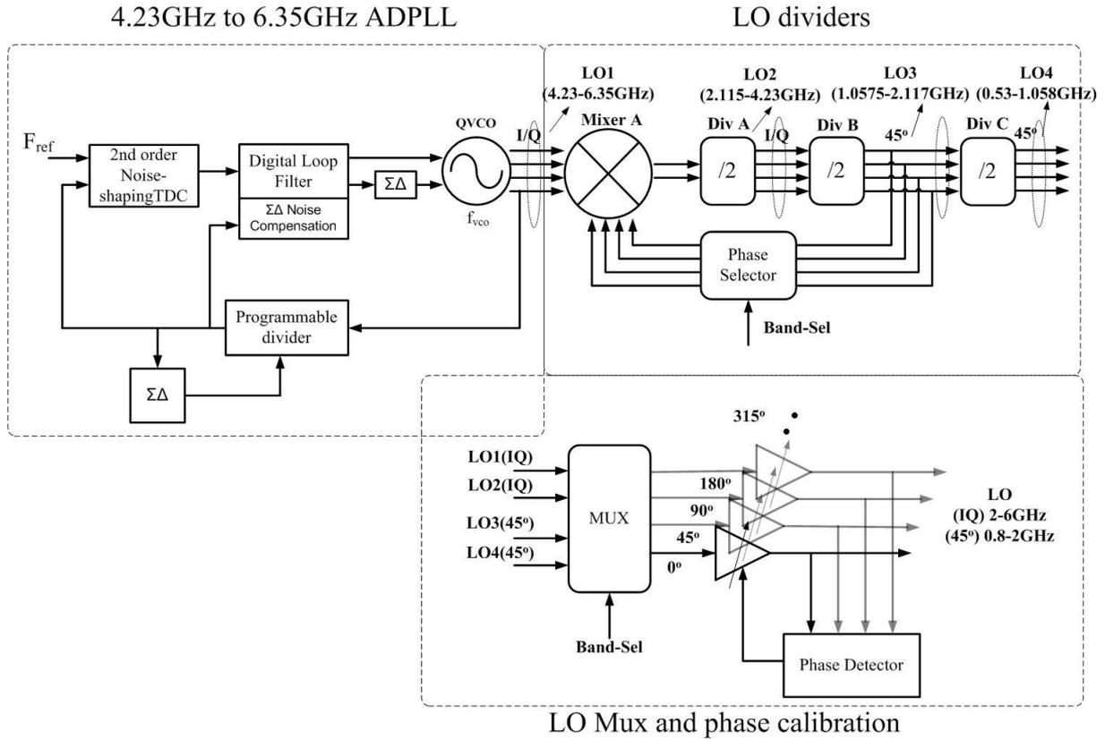
Fig. 1.9 Proposed ADPLL based frequency synthesizer
