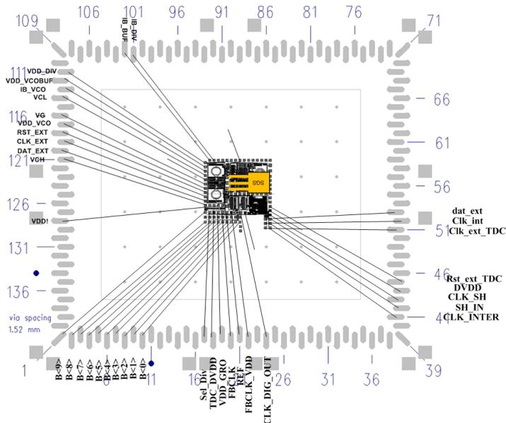
Fig. 6.25 An example of bonding diagram for the ADPLL
