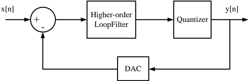
Fig. 5.11 Single-loop with higher-order loop filter
