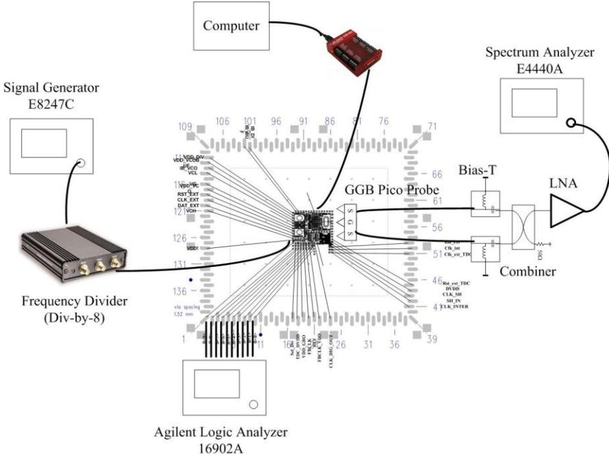
Fig. 6.26 Testing setup of the ADPLL
