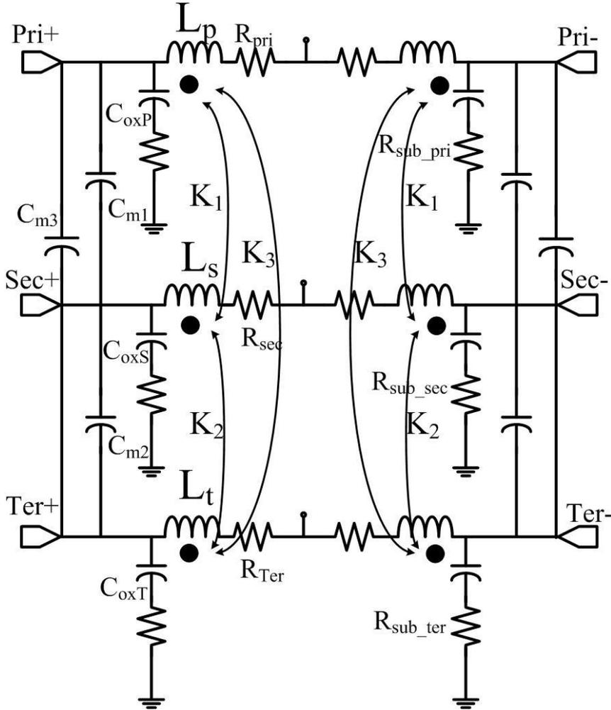
Fig. 8.8 3-coil transformer model for model fitting
