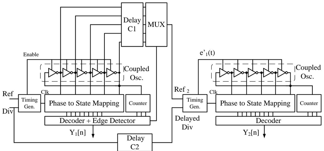
Fig. 5.14 shows the block diagram of the proposed 2<sup>nd</sup> order noise shaped TDC. The core
