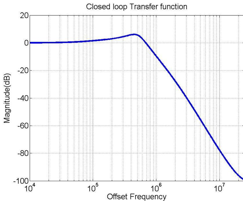
Fig. 5.8 ADPLL Closed-loop transfer function with  $LBW = 500kHz$  (TDC noise to output)
