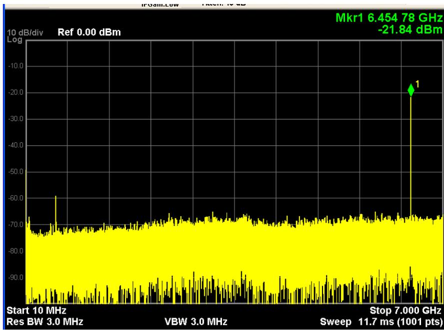
Fig. 8.9 Measured output spectrum of the LO with maximum output frequency @ 6.5GHz
