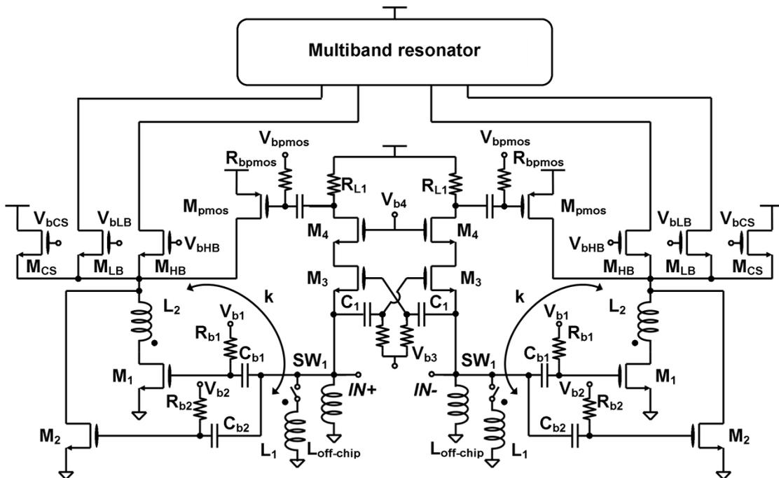
Fig. 7.1 Schematic of the SDR LNA
