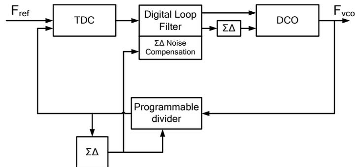
Fig. 6.2 Block diagram of a generic ADPLL
