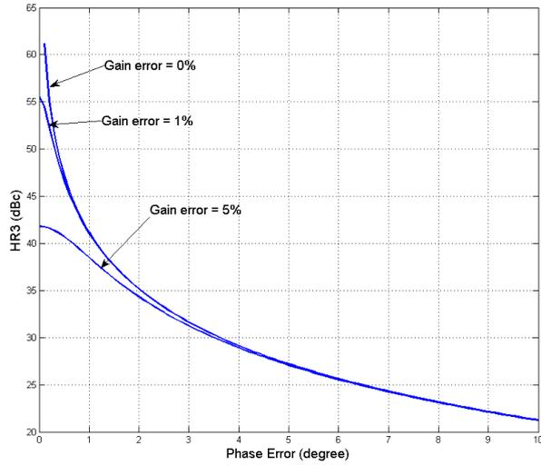
Fig. 3.9 Calculated HR3 as a function of phase error for various gain errors
