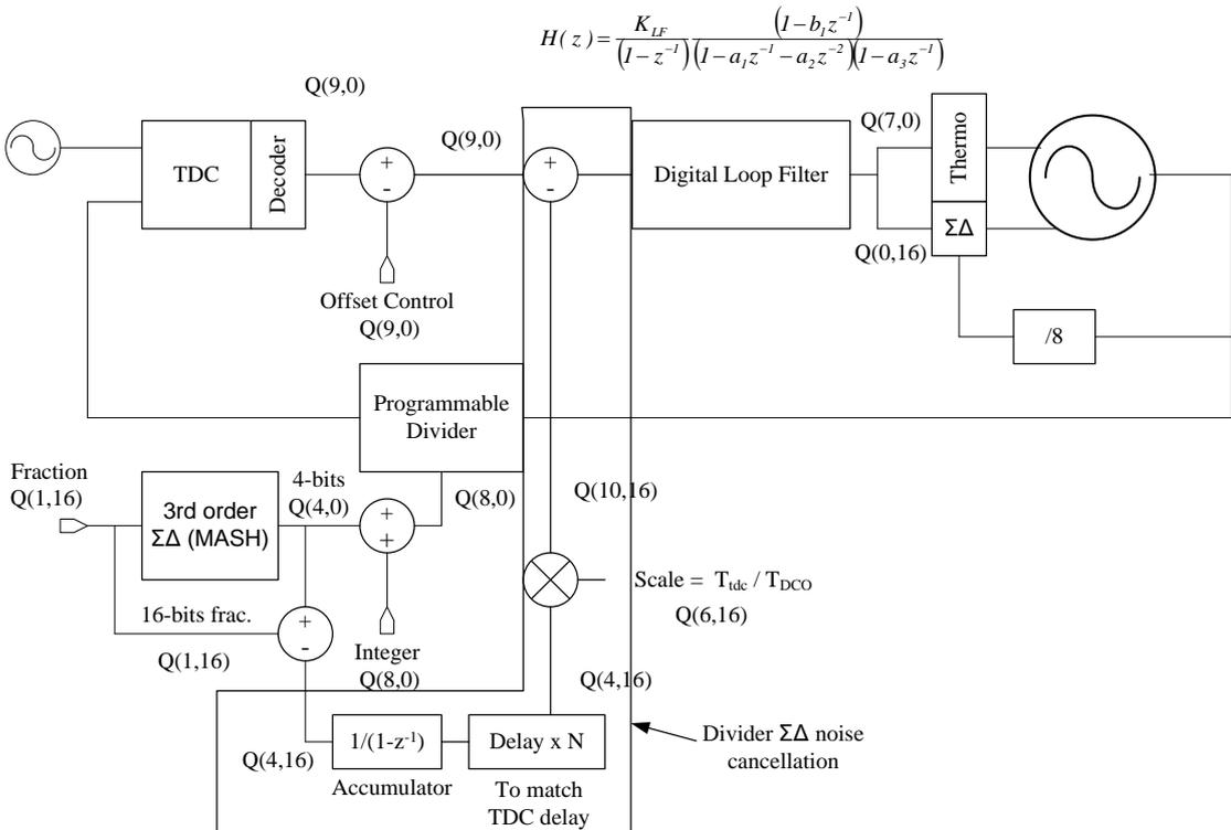
Fig. 6.10 shows a more detailed block diagram of the ADPLL system. The no. of bits of each digital signal line is indicated by Q(Integer, fraction). It is assumed every signal is in signed
