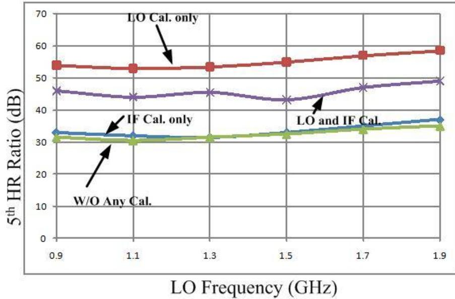
Fig. 8.21 Measured 5<sup>th</sup> order HR ratio (HRR mixer only) versus LO frequency
