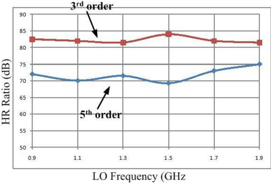
Fig. 8.22 Measured Total 3<sup>rd</sup> and 5<sup>th</sup> order HR ratio (RFE) versus LO frequency
