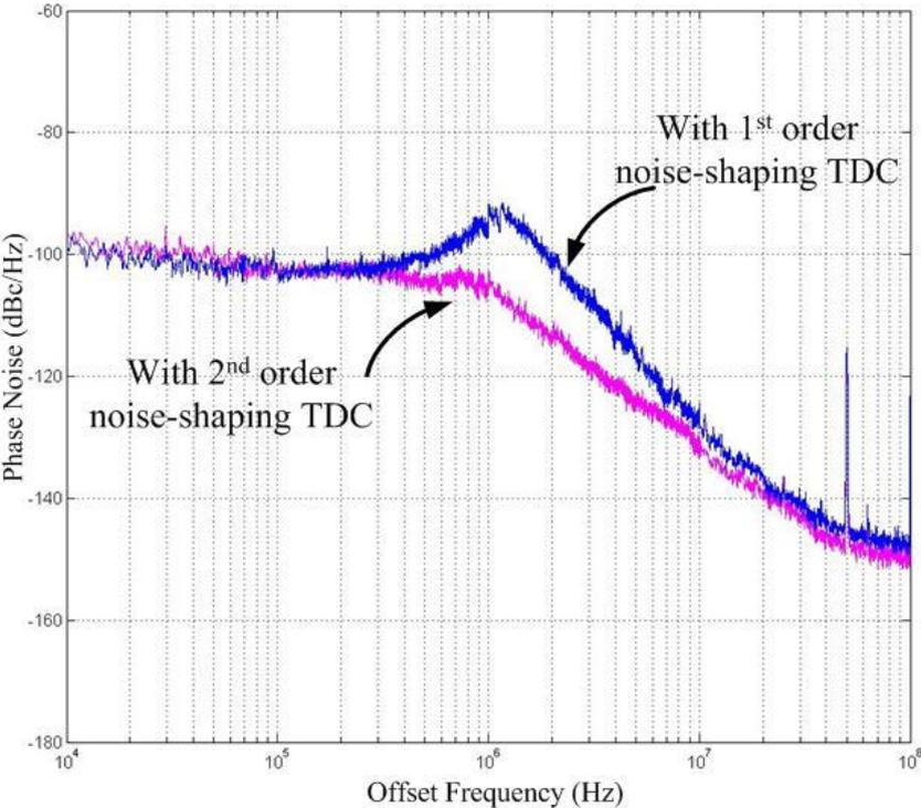
Fig. 6.34 Measured ADPLL phase noise with increased LBW (~1.2MHz)
