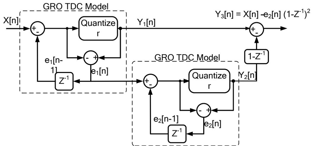
Fig. 5.15 Discrete-time model of the proposed TDC
