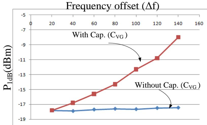
Fig. 8.16 Measured high-band  $P_{1dB}$  with RF located at  $f_{LO} + \Delta f$
