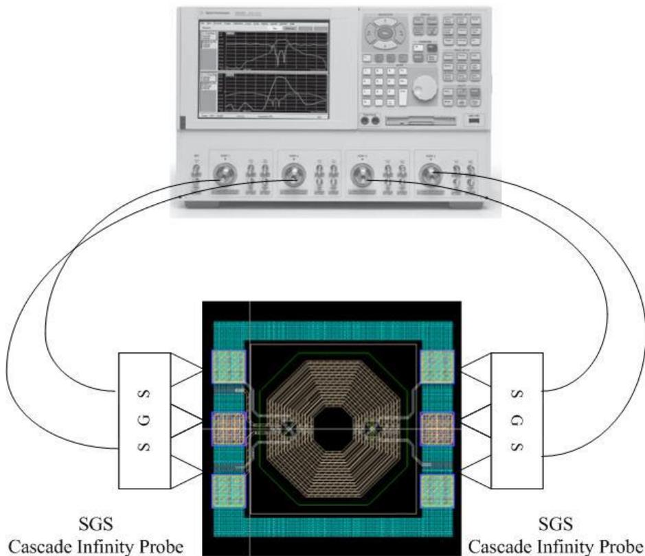
*Fig. 8.7 3-coil transformer S-parameter measurement*
