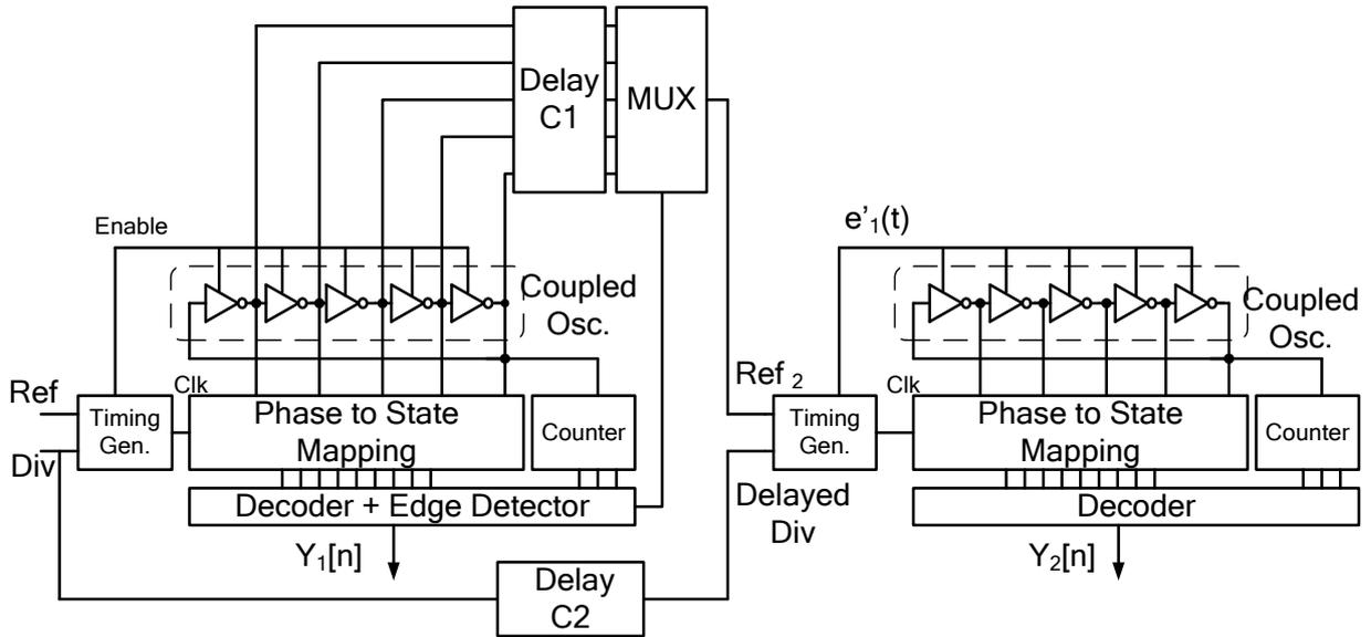
Fig. 5.14 Block Diagram of the 2<sup>nd</sup> order noise shaped TDC
