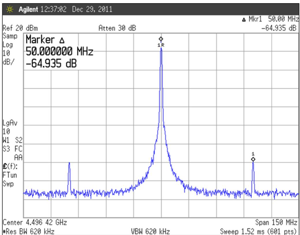
Fig. 6.28 Frequency spectrum of the ADPLL
