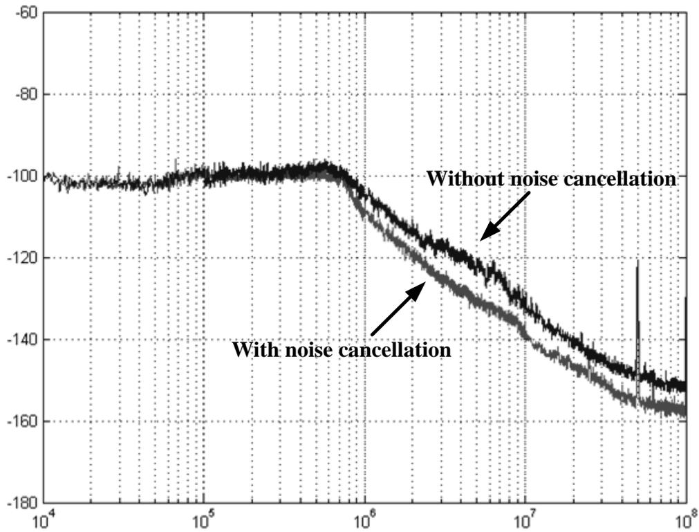
Fig. 6.30 shows the phase noise plot of the ADPLL with 2<sup>nd</sup> order noise-shaping with and without divider noise cancellation. As the figure reveals, greater than 10dB noise cancellation is achieved such that the out-of-band noise is dominated by the DCO. Fractional spurs are also tested with the spectrum analyzer as shown in Fig. 6.31, with -47.9 dBc.
