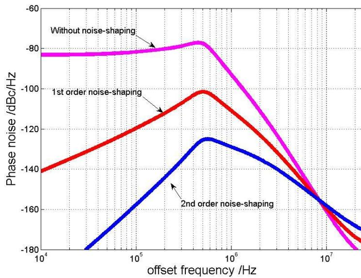
Fig. 6.8 TDC noise filtered by ADPLL Transfer function
