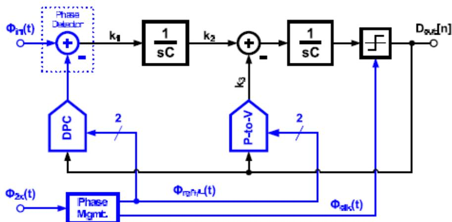
Fig. 5.34 Block diagram of a single-loop continuous-time  $\Delta\Sigma$  TDC [10]
