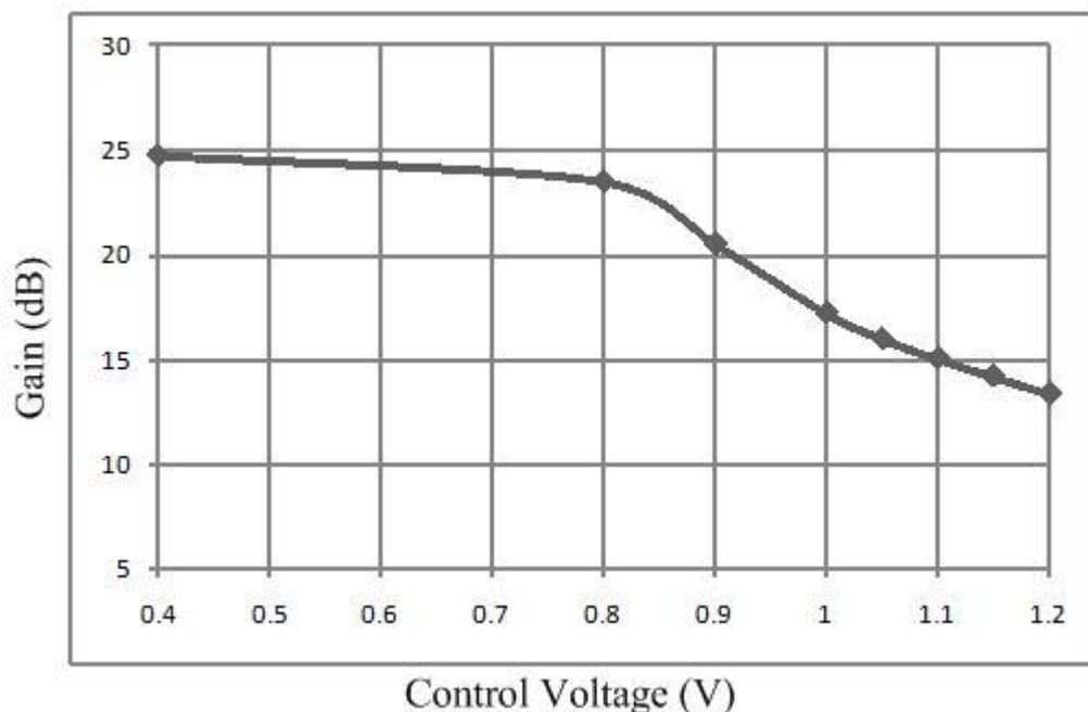
*Fig. 8.13 Measured Conversion gain vs control voltage*
