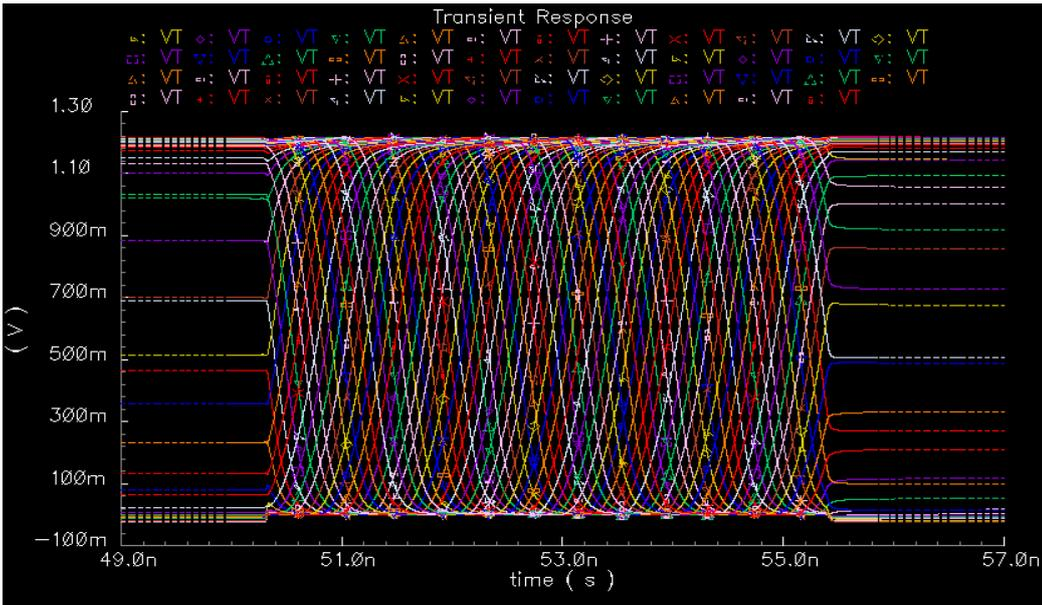
Fig. 5.21 Simulated waveform of the GRO during a time measurement
