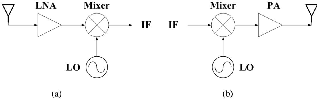
Fig. 2.5 Generic wireless transceiver (a) receiver front-end (b) transmitter
