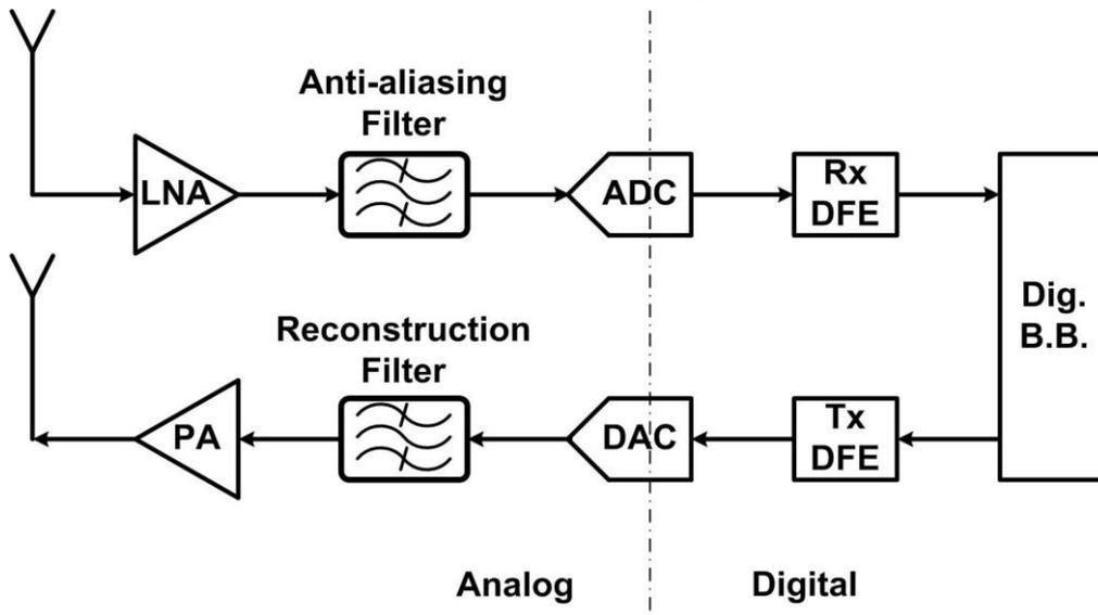
Fig. 1.2 Ideal SDR transceiver architecture
