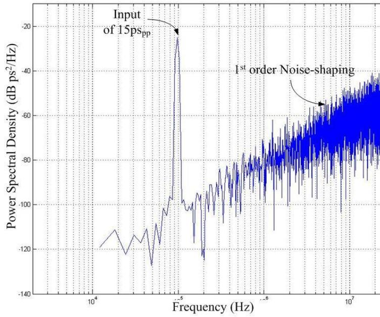
Fig. 5.28 Simulated 1<sup>st</sup> order TDC PSD without GRO phase noise with 60ps resolution
