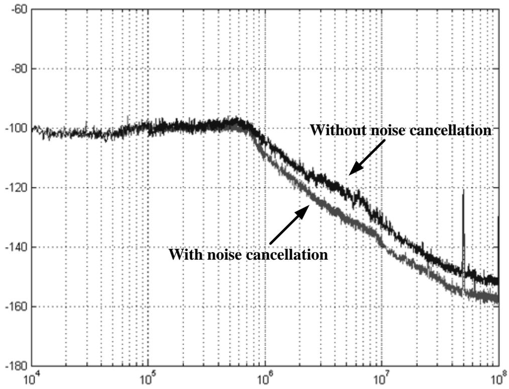
Fig. 6.30 Measured Phase noise plot with and without divider noise cancellation
