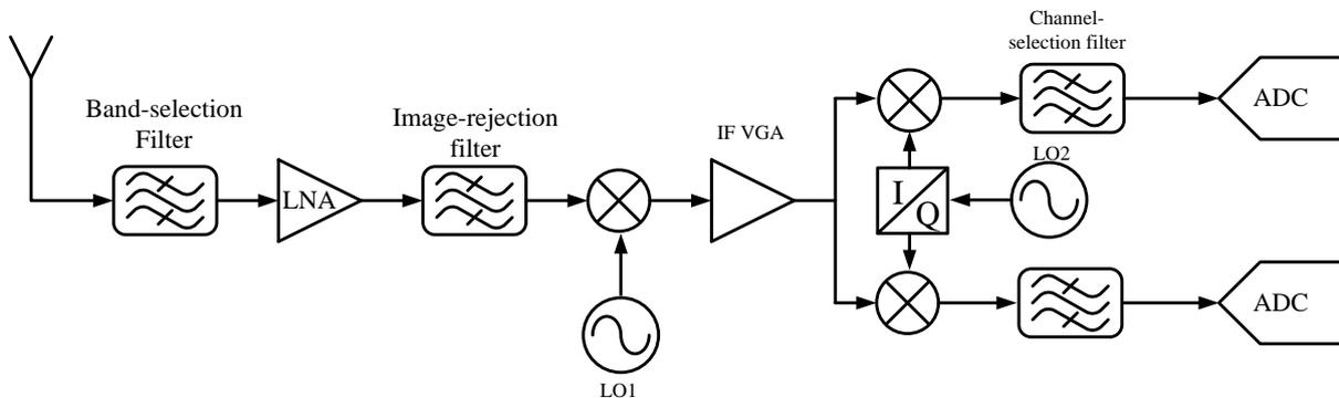
Fig. 3.3 Super-heterodyne receiver
