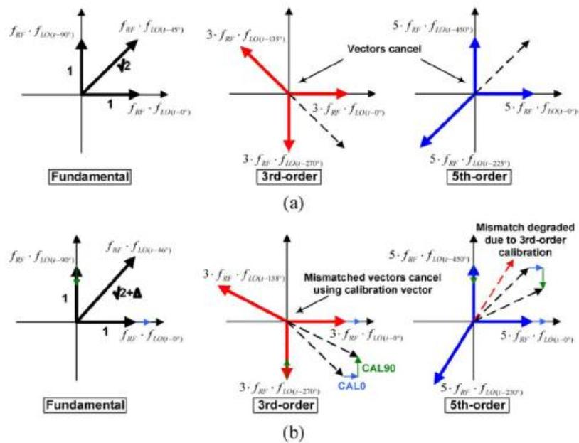
Fig. 3.13 Vector phase sum diagram: (a) without mismatch and (b) with gain and phase mismatch [8]
