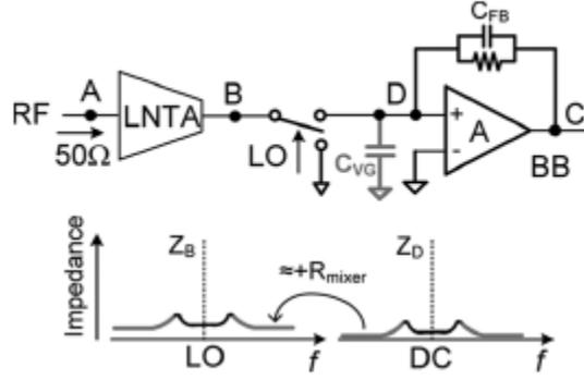
Fig. 3.16 Illustration of impedance transfer
