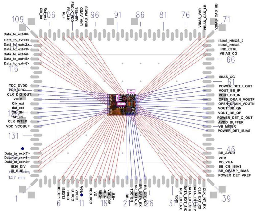
Fig. 8.3 Bonding Diagram for the proposed SDR RFE
