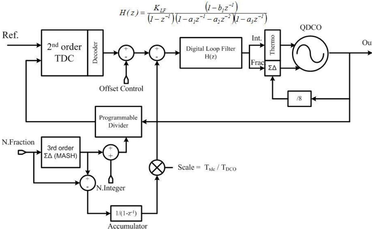
Fig. 6.16 System block diagram of the ADPLL Frequency Synthesizer
