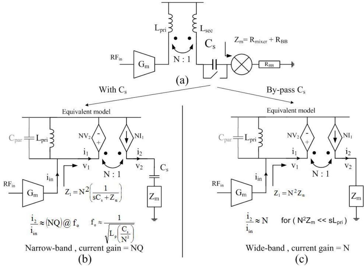
Fig. 4.1 Transformer-based current-gain-boost technique (a) Block diagram (b) Equivalent model with  $C_s$  (c) Equivalent model by-passing  $C_s$
