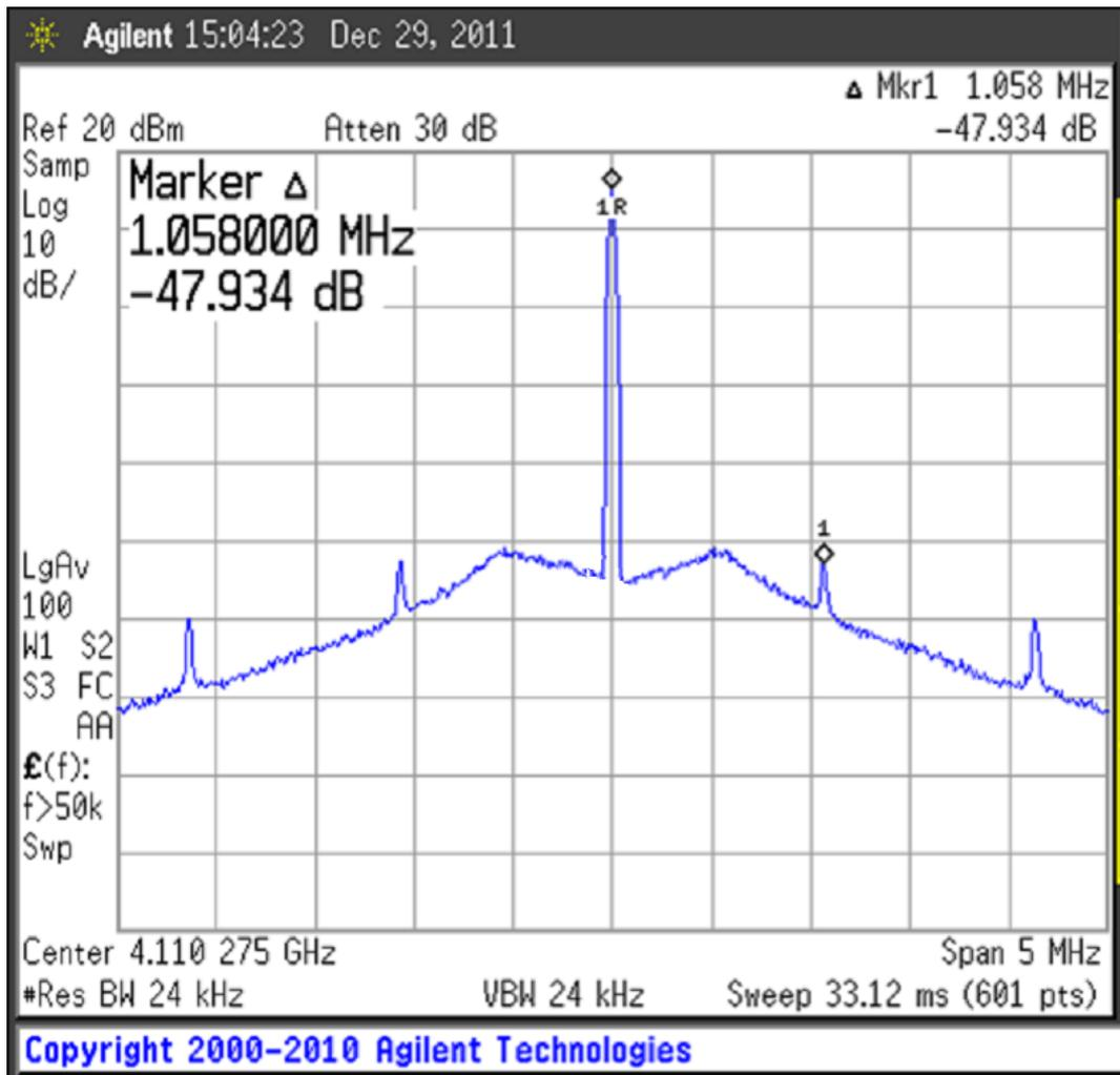
Fig. 6.31 Measured fractional spur of the ADPLL
